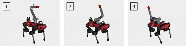
(a) 1. Robot starts in a nominal stance mode. 2. Base is commanded to roll with a 30 degree angle. 3. Left fore leg is lifted.
