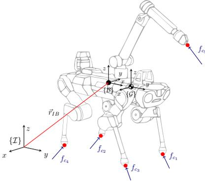
Fig. 2: Illustration of the multi-limbed floating-base system used in this work. The sketch depicts the main reference frames used in our derivation of the equations of motion (inertial  $\{I\}$ , base  $\{B\}$ , and centroidal  $\{G\}$  frames), in addition to the contact forces acting on the limbs.
