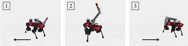
(b) 1. Robot is trotting laterally in one direction. 2. Robot is commanded to switch directions. 3. Robot is trotting laterally in the other direction.
