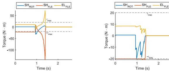
Fig. 6: Plots showing the arm’s joint torques for the dynamic throwing task without torque limits (*left*) and with torque limits (*right*)
