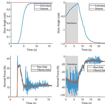
Fig. 8: Plots showing the estimated door angle and the normal force applied to the door for the pushing (*left*) and pulling (*right*) experiments. The door is disturbed during the pulling task.
