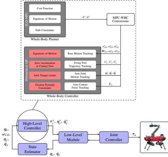
Fig. 3: A schematic diagram depicting the various components of the full control architecture. The high-level control module is highlighted and detailed in the top diagram. This consists of the whole-body planner interacting with the WBC whose high-priority tasks are indicated in red.
