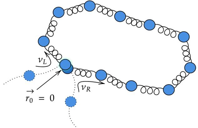
FIG. 1. Growth of polymer loop via two sided extrusion process. The extrusion velocities  $v_L = \frac{1-q}{2}v_0$  and  $v_R = \frac{1+q}{2}v_0$  represent the rates at which the LEF adds new beads at the left and right arm of the loop, respectively, and  $q$  is the so-called symmetry score introduced in Ref [8]. The choice  $q = 1$  corresponds to the pure one-sided extrusion, while at  $q = 0$  we deal with perfectly symmetric two-sided loop growth.
