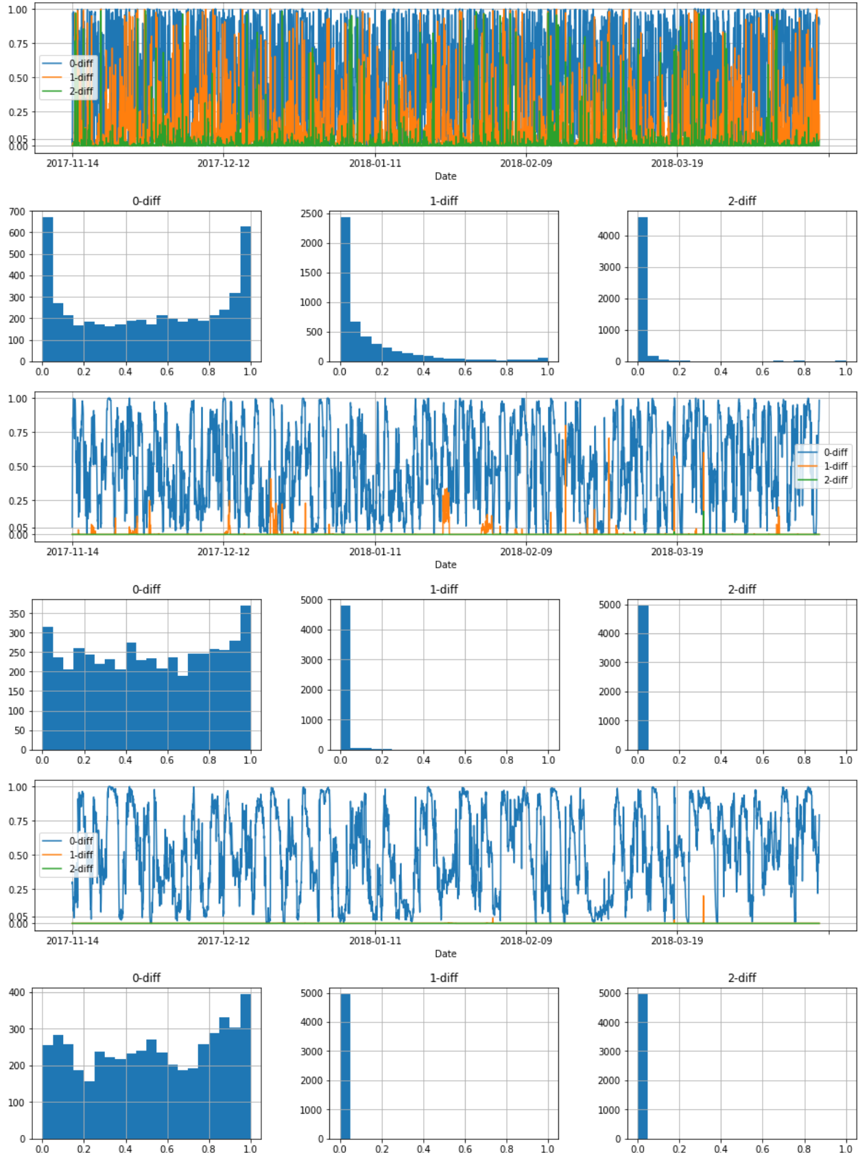
Figure 3: Results from rolling ADF tests for different window sizes: 12 (top two), 48 (centre two), and 96 (bottom two).
