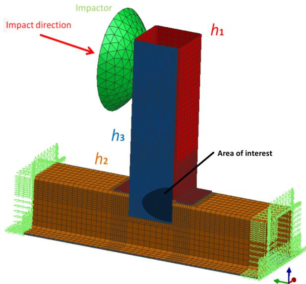
Figure 1 Crash benchmark. Thicknesses  $h_1$ ,  $h_2$  and  $h_3$  are the three input random parameters corresponding to the vertical profile (red), horizontal profile (orange) and plate profile (blue). The impactor (green), and the area of elements of interest (black) are also depicted.
