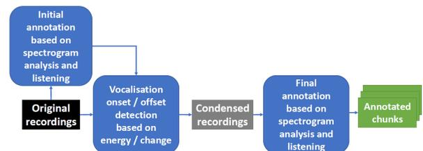
Figure 1: The semi-automatic annotation pipeline used in the study.
