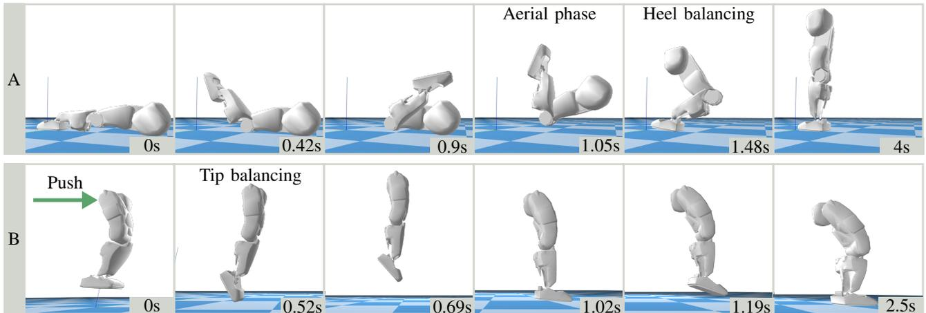
Fig. 5. Time-lapse snapshots of contact-rich motions: (A) Standing-up from ground by a dynamic manoeuvre using large momentum with aerial phases. (B) Robust balancing by toe tipping and jumping that withstands an external push.
