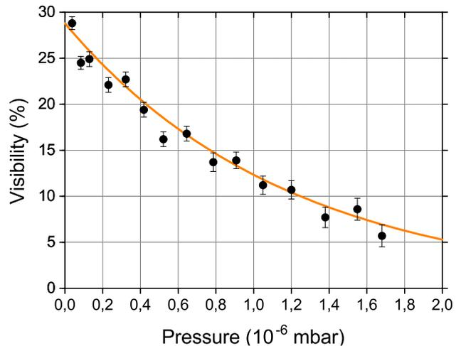
FIG. 4. Reduction of the interference visibility of  $C_{70}$  molecules in a TLI due to collisions with the background gas (argon) as a function of gas pressure. The data is in excellent agreement with the expected exponential loss of contrast (solid line). (Reproduced from Ref. [48])
