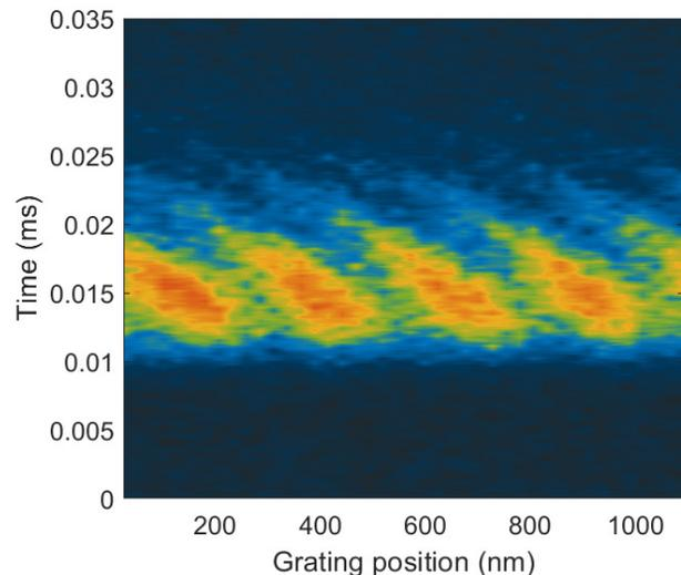
FIG. 1. Matter-wave fringes in fullerene interferometry for different flight times of  $\text{C}_{60}$  molecules through the LUMI interferometer (with grating period 266 nm). The Coriolis force entails a velocity dependence of the phase of the interference fringes. The phase difference between fast and slow molecules can easily exceed  $2\pi$ . (Reproduced from Ref. [32])
