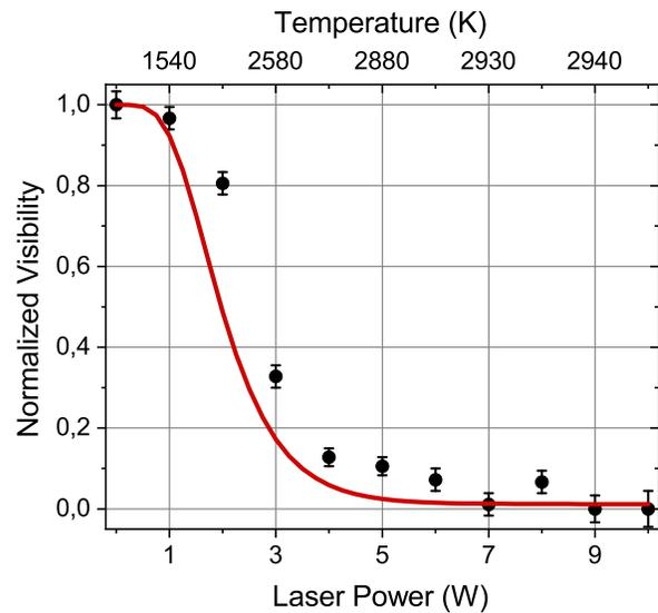
FIG. 6. Loss of visibility due to thermal decoherence plotted versus heating power (lower scale) and mean internal temperature of the  $C_{70}$  molecules when they enter the Talbot-Lau interferometer (upper scale) at a mean velocity of  $v_m = 100\text{ m/s}$ . (Reproduced from Ref. [46])
