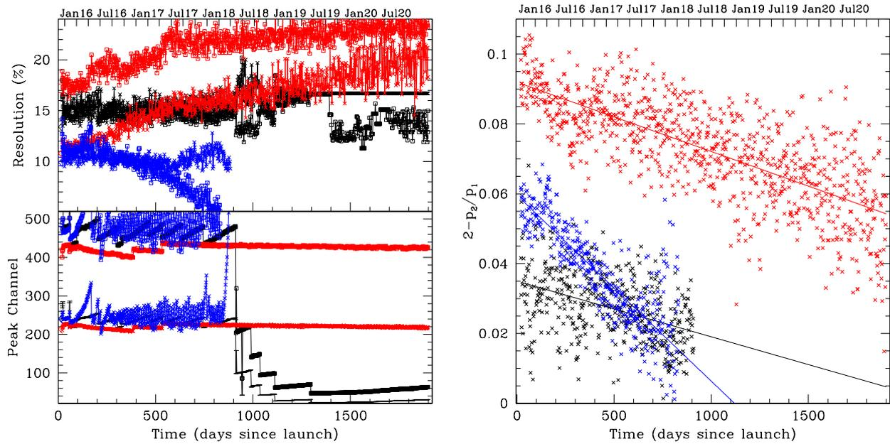
**Figure 2.** The energy resolution and peak channel for the 30 keV ( $p_1$ , as marked by cross) and 60 keV ( $p_2$ , as marked by open squares) calibration peak in veto anode A8 is shown in the left panel. The black, red and blue points show the result for LAXPC10, LAXPC20 and LAXPC30, respectively. The right panel shows the quantity  $2 - p_2/p_1$  for the three detectors. The lines mark the best fit straight lines for the three detectors.
