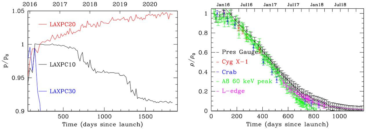
**Figure 1.** The pressure in LAXPC detectors as a function of time. The left panel shows the pressure as obtained from the pressure gauge for all three detectors. The right panel shows the density for LAXPC30 using various techniques. The dashed-line is the fit to linear part of the curve. Both pressure and density are shown relative to their initial values.
