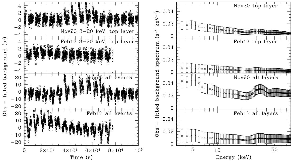
**Figure 14.** The residuals in the fit to background of LAXPC20 for the two background observations obtained using the background model described by Antia et al. (2017). The left panel shows the residuals in the light curve with a time-bin of 32 s, while the right panel shows the residuals in the energy spectrum.
