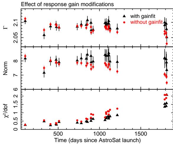
**Figure 5.** The results of fit to Crab spectrum observed by LAXPC20 during the last 5 years is shown as a function of days from launch of AstroSat. The results with and without applying the `gain fit` are shown.
