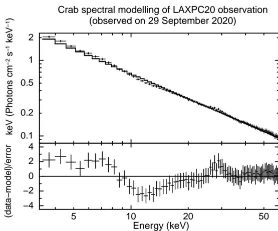
**Figure 6.** A fit to the Crab spectrum observed by LAXPC20 during September 2020 to powerlaw model with `gain fit` is shown. The lower panel shows the residuals. The reduced  $\chi^2$  of the fit with 3% systematics is 2.03.
