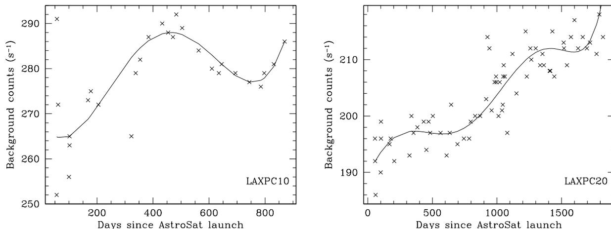
**Figure 10.** The total count rate in background corrected for gain shift as a function of time for LAXPC10 and LAXPC20.
