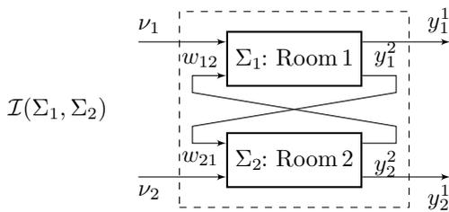
FIGURE 18. Interconnection of two rooms  $\Sigma_1$  and  $\Sigma_2$ .
