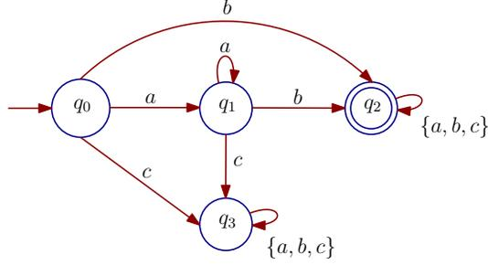
FIGURE 5. DFA  $\mathcal{A}_\varphi$  of the reach-avoid specification  $(a \text{ U } b)$ .
