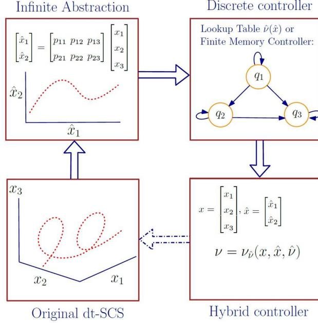
FIGURE 7. **Infinite abstractions.** The original dt-SCS has a 3-dimensional state set while its abstraction has a 2-dimensional state set. This model reduction can be performed via a transformation matrix  $P$  satisfying conditions (4.4) and (4.5).
