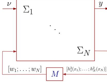
FIGURE 15. An interconnected dt-SCS with external input and output signals  $\nu$  and  $y$ , respectively. Note that in so-called small-gain settings discussed later, the interconnection matrix  $M$  is a permutation matrix that results in an element-wise interconnection constraint (i.e.,  $\forall i, j \in \{1, \dots, N\}, i \neq j: w_{ij} = h_{ji}^2(x_j)$ ).
