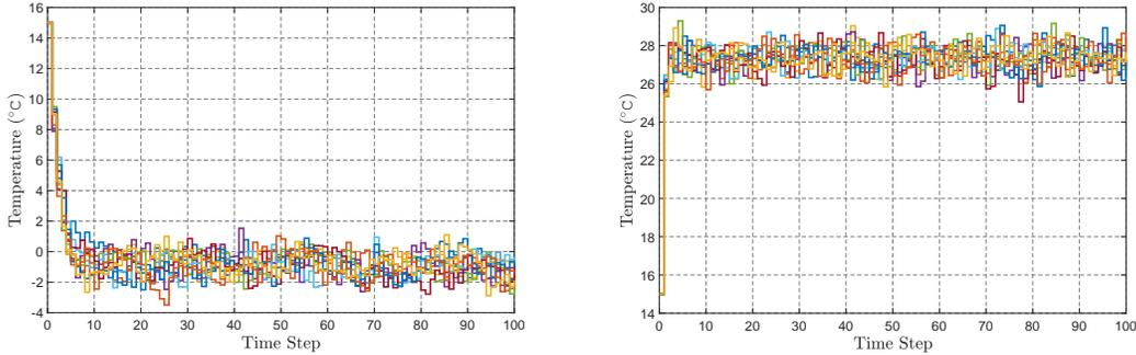
FIGURE 4. State trajectories, generated for the running example with 10 different noise realizations within the finite time horizon  $T_d = 100$  from an initial condition  $x_0 = 15$ , and with  $\nu = 0$  (top, heating off) and  $\nu = 1$  (bottom, heating on), respectively.
