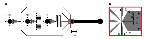
**Figure 1. Microfluidic chip design. a)** Outline of the microfluidic device. OA, MO and IA indicate inlets for the outer aqueous, middle organic and inner aqueous phases respectively. **b**) Magnified view of the flow focusing junction indicating important dimensions.
