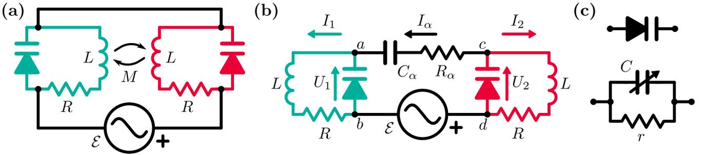
Figure 1. The system under the consideration: two coupled RLC circuits driven by the harmonic source. Coupling between the circuits may be introduced in different ways as (a) and (b) demonstrates. (c) Equivalent scheme of the varactor diode, which consists of the capacitor  $C$ , series resistance  $R$  and resistance elements  $r$  and  $R$ .
