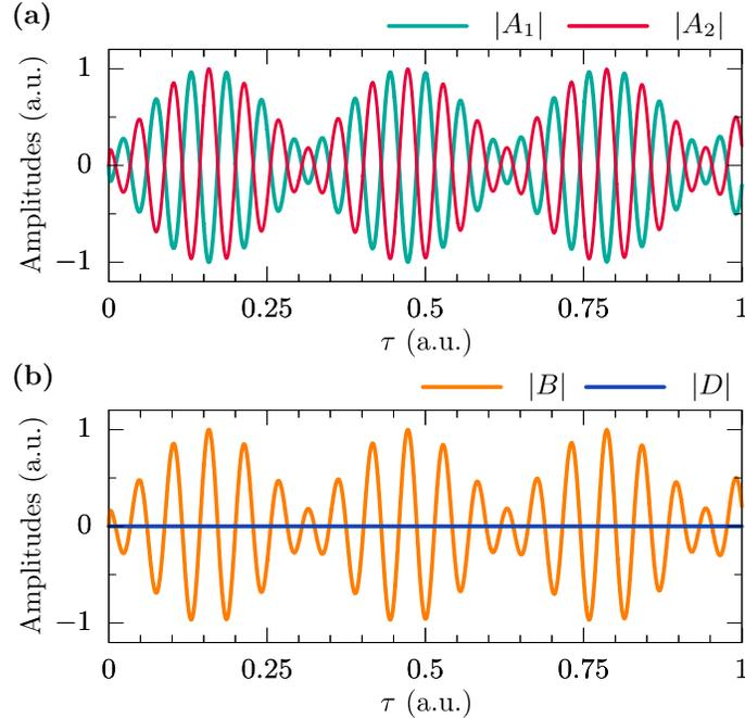
Figure 2. (a) Voltage oscillations in considered RLC circuits and (b) their interference representing the normal modes of the system.
