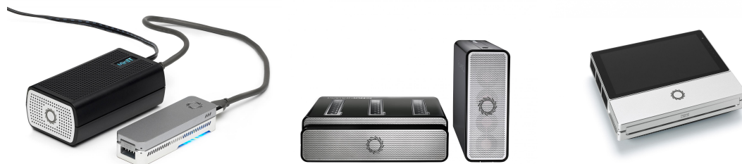
(a) MinION sequencer (right) connected to the MinIT base-calling unit (left) (b) PromethION sequencer (right) and its compute tower with integrated base-calling unit (left) (c) MinION Mk1C sequencer
