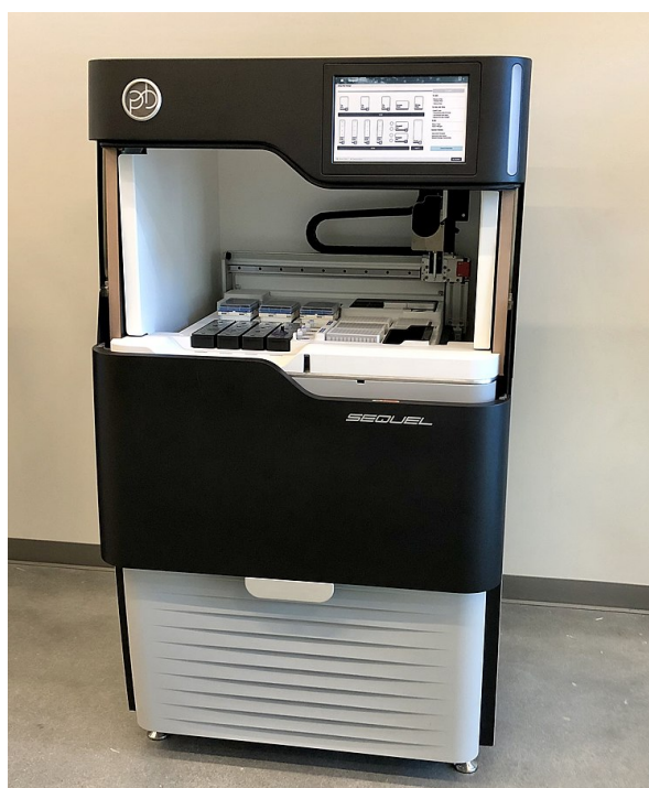
Figure 2.9: Pacific Biosciences Sequel Sequencer. Photograph from https://en.wikipedia.org/wiki/File:SequelSequencer.jpg licensed under CC BY-SA 4.0. Dimensions are 92.7 x 86.4 x 167.6 cm
