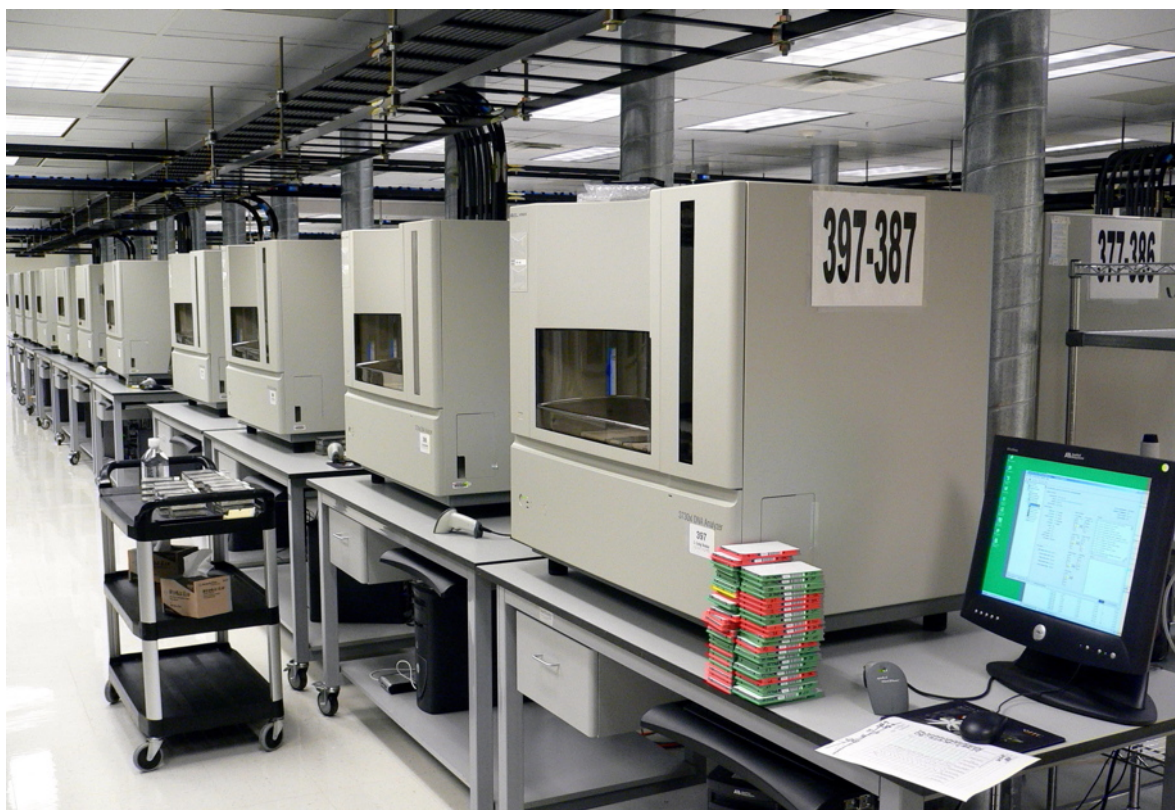
Figure 2.7: First-generation sequencers. A row of Applied Biosystems 3730xl DNA Analyzer machines. Photo is from [47] licensed under CC BY 2.0. The weight of a machine is 180 kg and the dimensions are 100 cm (W) x 73 cm (D) x 89 cm (H) [48].
