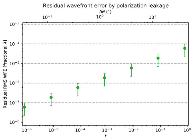
**Fig. 10.** Performance of the wavefront sensing with polarization leakage. The error bars show the  $1\sigma$  deviation over the 100 random wavefront aberration instances. The bottom x-axis shows polarization leakage ( $t$ ), and the upper x-axis shows the equivalent rotation offset ( $\delta\theta$ ) between the RH polarizer and PBS. We note that the right most data point is sampled at  $t = 0.81$ .
