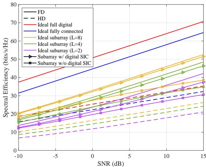
Fig. 6. Digital SIC ability of a 4-user wideband mmWave-FD-IAB subarray network in terms of different numbers of RF chains ( $L = 2, 4, 8$ ) on each Rx subarray. Equipped with  $16 \times 16$  UPA on both sides, 4 RF chains at Tx and 4 data streams are transmitted.
