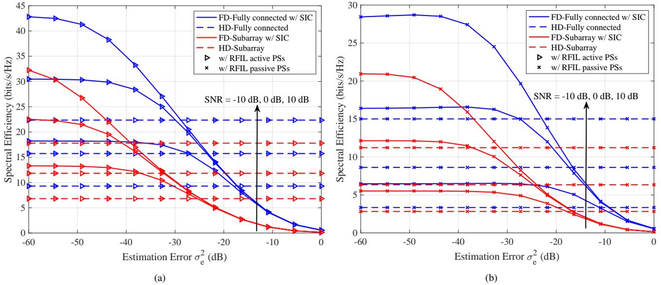
Fig. 5. Comparison of the impact of CEE on the backhaul link SE in the presence of RFIL of a 4-user mmWave-FD-IAB system with different hybrid precoding structures in terms of different SNR values. Equipped with  $16 \times 16$  UPA, 4 (8) RF chains at Tx (Rx), 4 data streams are transmitted. The number of subarrays is equal to that of the user: a) with active PSs; b) with passive PSs.
