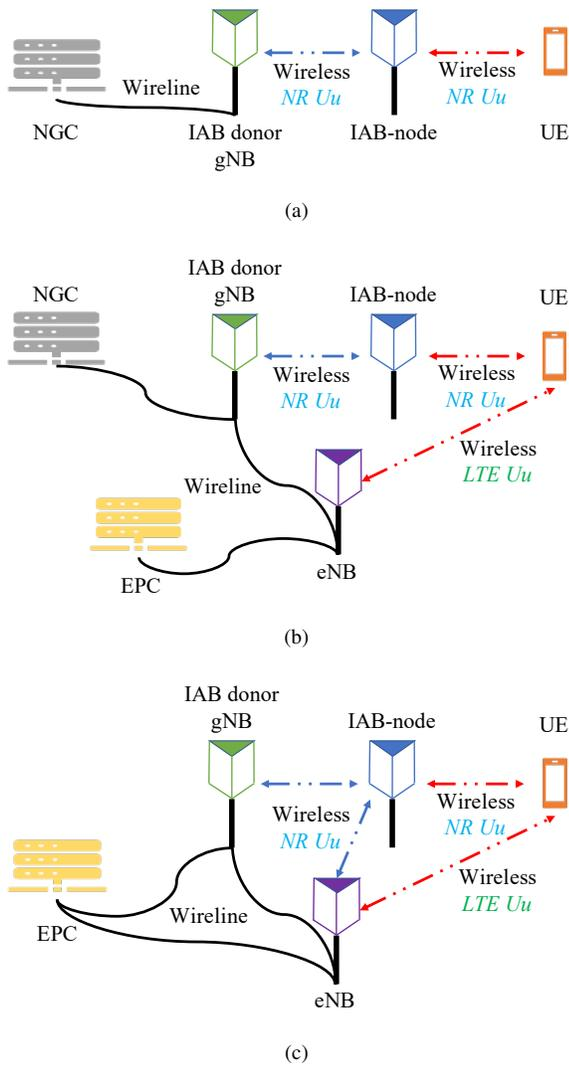
Fig. 1. Examples for FD-IAB network architectures operating in SA mode and NSA mode: a) UE: SA with NGC, IAB node: SA with NGC; b) UE: NSA with EPC, IAB node: SA with NGC; c) UE: NSA with EPC, IAB node: NSA with EPC.
