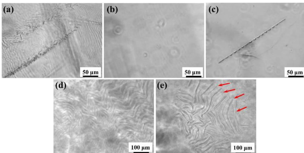
**Figure 3.** Optical images of hydrogel C2-40 following either 3-week incubation in  $\text{Na}_2\text{HPO}_4$  (a), PBS (b), and c-SBF (c), or 3-month incubation in PBS buffer (d and e). Deep aggregation of the network was indicated with red arrows.
