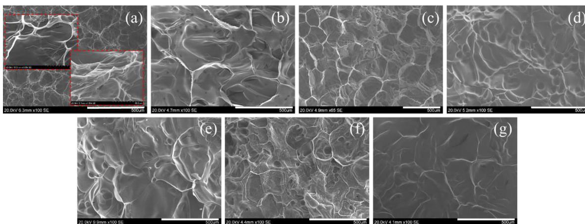
**Figure S5.** SEM images of freeze dried E2-40 networks following 4-week incubation in (NH<sub>4</sub>)<sub>2</sub>SO<sub>4</sub> (a), Na<sub>2</sub>SO<sub>4</sub> (b), Na<sub>2</sub>HPO<sub>4</sub> (c), NaAc (d), NaCl (e), PBS (f) and deionized water (g). Scale bar: 500 μm.
