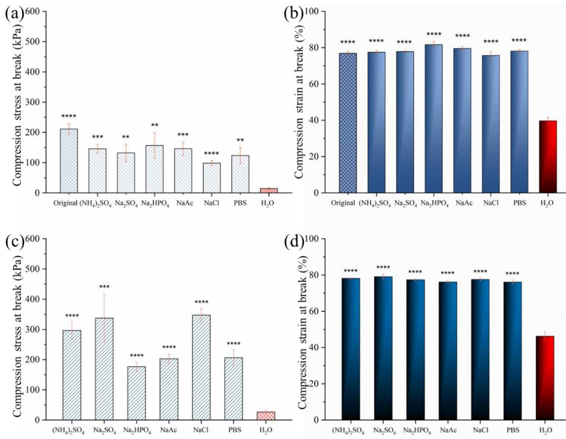
**Figure S4.** Compression measurements of hydrogel E2-40 after synthesis ('Original') and following 1-day (a, b) and 4-week (c, d) incubation in different aqueous solutions. All the statistical analysis is presented with respect to the H<sub>2</sub>O group and labelled as \*\*p < 0.01, \*\*\*p < 0.001, \*\*\*\*p < 0.0001. All the data are presented as Mean±SD.
