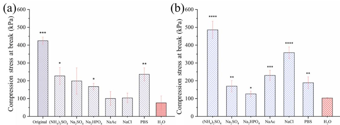
**Figure S3.** Compression stress at break of hydrogel C2-40 measured after synthesis ('Original') and after 1-day (a) and 4-week (b) incubation in different aqueous solutions. All the statistical analysis is presented with respect to H<sub>2</sub>O group and labelled as \*p < 0.05, \*\*p < 0.01, \*\*\*p < 0.001, \*\*\*\*p < 0.0001. All the data are presented as Mean±SD.
