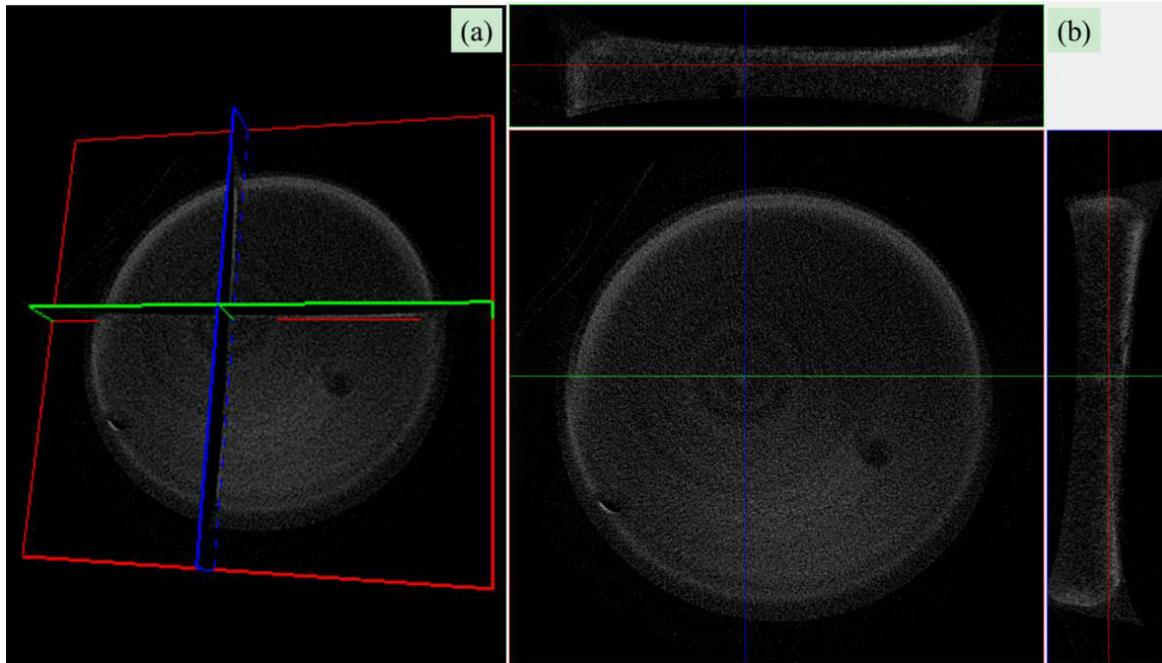
**Figure S11.** Macro-pattern study of mineralized sample C2-40 from  $\mu\text{CT}$  scan, combining 3-dimensional image (a) and cross section of each axis (b).
