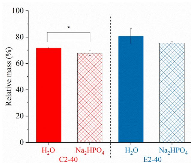
**Figure S2.** Relative mass of hydrogels (n=4) C2-40 (red) and E240 (blue) after 4-week immersion in either the Na<sub>2</sub>HPO<sub>4</sub>-supplemented solution (50 mM) or deionised water.
