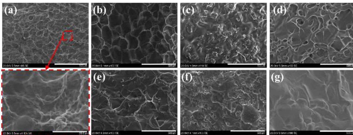
**Figure 2.** SEM images of freeze-dried C2-40 networks following 4-week incubation in aqueous solutions. (a):  $(\text{NH}_4)_2\text{SO}_4$  (including zoomed-in image below); (b):  $\text{Na}_2\text{SO}_4$ ; (c):  $\text{Na}_2\text{HPO}_4$ ; (d):  $\text{NaAc}$ ; (e):  $\text{NaCl}$ ; (f):  $\text{PBS}$ ; (g):  $\text{H}_2\text{O}$ . Scale bar of (a-g):  $500\ \mu\text{m}$ . Scale bar of zoomed-in image of (a):  $50\ \mu\text{m}$ .
