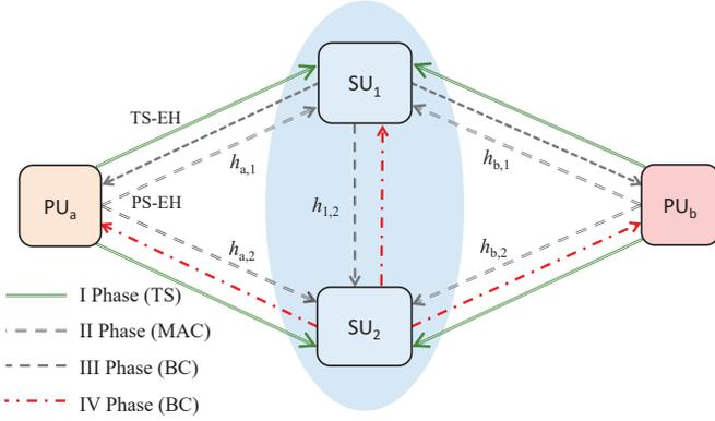
Fig. 1. System model for hybrid TS/PS SWIPT in cognitive radio networks.
