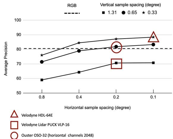
FIGURE 3. The average precision for detecting vehicles from depth data at different spatial resolutions. The lines connect simulations at a common vertical resolution, and the x-axis measures horizontal resolution. The red symbols indicate the spatial resolution of different commercial sensors. The performance using data from an RGB camera ( $1920 \times 650$ ) is shown by the horizontal dashed line.
