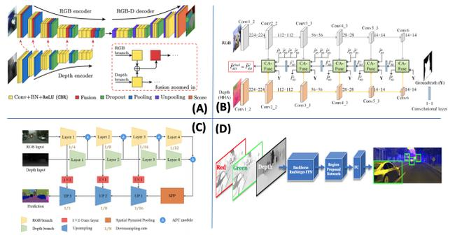
FIGURE 12. Sensor fusion architectures. Panels (A-C) are overviews of the network architectures from three different papers that fused radiance and depth images. Panel (D) is the ResNet architecture used in this paper that uses RGD as the fused input. (A) (Copied from Hazirbas et al., 2016) [15] (B) (Copied from Chen et al.2018) [3] (C)(Copied from Sun et al.2020) [25] (D) Ours: RGD.
