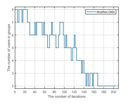
Fig. 5. The number of users in MOMA clusters different from the optimal partitioning under increased number of iterations (The number of users is 8).
