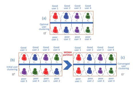
Fig. 3. The MOMA based user clustering (number of users is 8). The users are divided into two groups. (a) presents the optimal user clustering where good user 1 and poor user 1 constitute a NOMA group. (b) shows the initial user clustering which is not an optimal solution. (c) illustrates the converged user clustering of the proposed MOMA algorithm.
