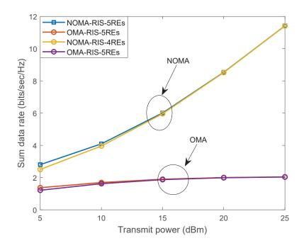
Fig. 8. The sum data rate versus the AP transmit power.
