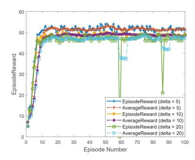
Fig. 6. The sum reward versus the number of trials for different delta (delta represents the granularity in the action space for changing the phase shifts of the RIS).
