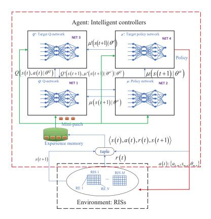
Fig. 4. The framework of the proposed DDPG algorithm for RIS-aided NOMA downlink transmission.
