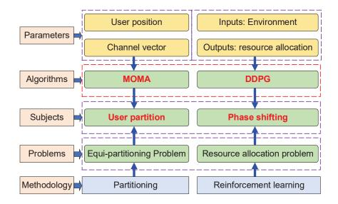
Fig. 2. The proposed MOMA and DDPG algorithm for user clustering and phase shifter design of the RIS. The users are partitioned into equal-size clusters by the proposed MOMA algorithm. The REs of the RIS are controlled by the intelligent agent of the DDPG algorithm, who is capable of learning the optimal phase shifts through exploration and exploitation.
