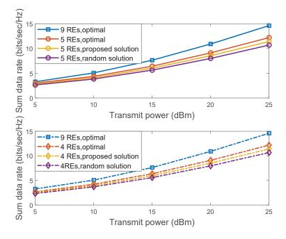
Fig. 7. The sum data rate versus the AP transmit power.
