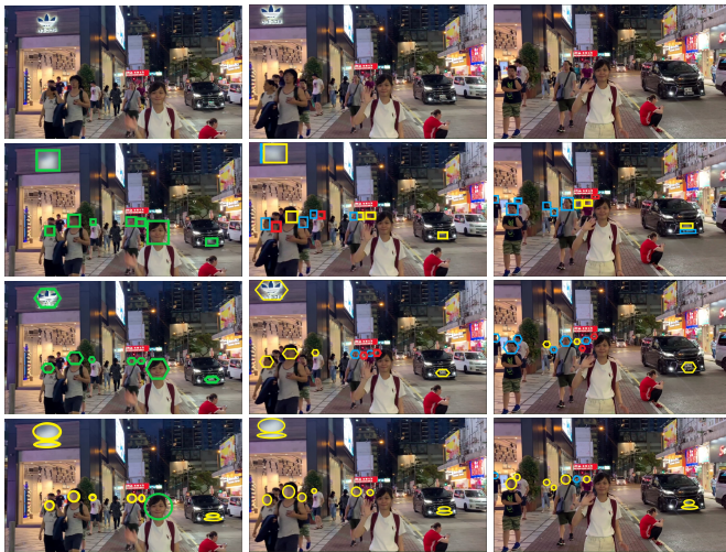
Figure 3: Qualitative comparison of YouTube (mosaics in rectangular), KCF (mosaics in hexagons), and PsOP (mosaics in circles). Green boxes indicate human intervention is needed for specification, yellow are the auto-generated mosaics, red ones are the over-pixelated area, and blue ones are the miss-pixelated area.
