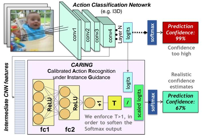
Fig. 3: Overview of the Calibrated Action Recognition under Instance Guidance Model (CARING). CARING is an additional neural network which learns to infer the scaling factor  $\mathcal{T}$  depending on the instance representation. The logits of the original activity recognition network are then divided by  $\mathcal{T}$ , giving better estimates of the model uncertainty.
