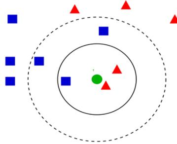
**Fig. 7** Euclidean Distance Measurement
