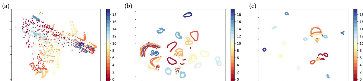
Figure 1: Comparison of different dimensional reduction algorithms on Coil 20 dataset. Total 20 different labels are in the Coil 20 dataset, and we use the ground truth label to color each data points. (a) Feature size is reduced to dimension 2 by PCA. (b) Feature size is reduced to dimension 2 by t-SNE. (c) Feature size is reduced to dimension 2 by UMAP.
