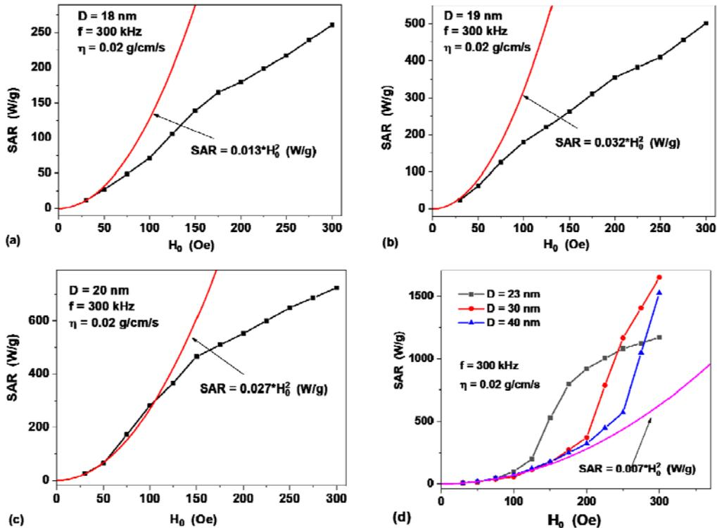
Fig. 4. Dependence of the SAR of a dilute assembly in a liquid (dots) on the magnetic field amplitude for particles of different diameters: a)  $D = 18$  nm, b)  $D = 19$  nm, c)  $D = 20$  nm and d)  $D = 23-40$  nm. The solid curves are drawn in accordance with Eqs. (1) - (3).
