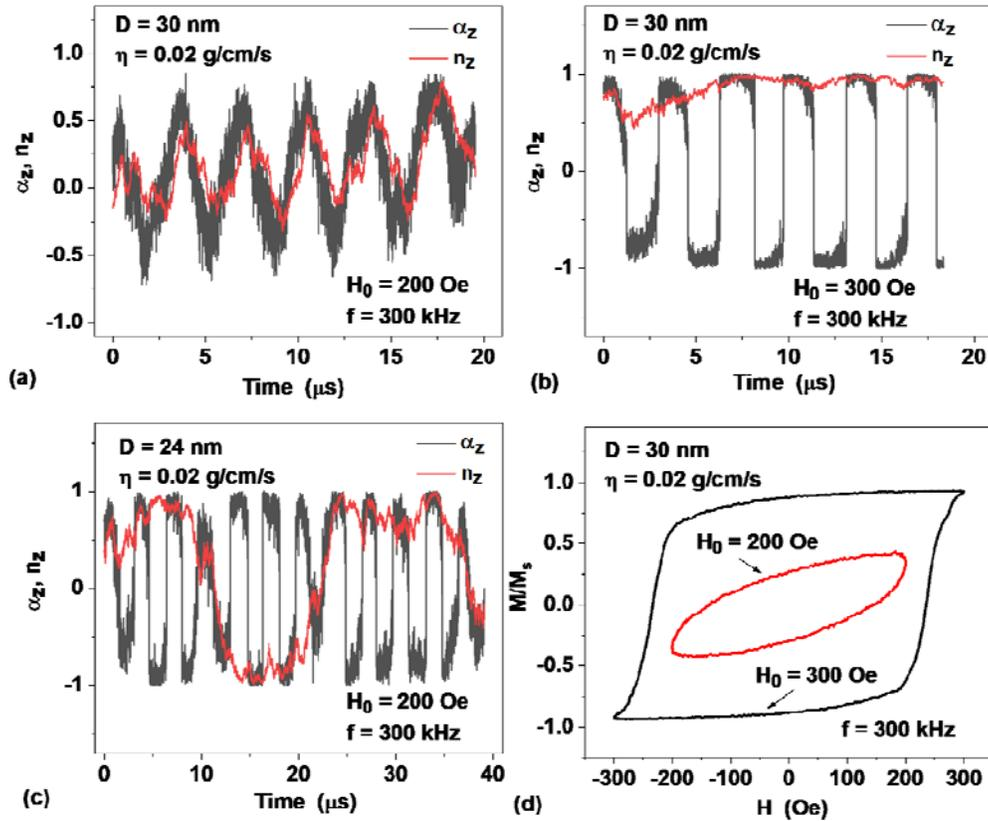
Fig. 2. The nature of the motion of the unit magnetization vector and director of an individual nanoparticle of the assembly in a viscous liquid for different cases: a) developed viscous mode, point 1 in Fig. 1a, b) developed magnetic mode, point 2 in Fig. 1a, c) intermediate regime, point 3 in Fig. 1a. d) low frequency hysteresis loops for viscous and magnetic modes at points 1 and 2 in Fig. 1a, respectively.
