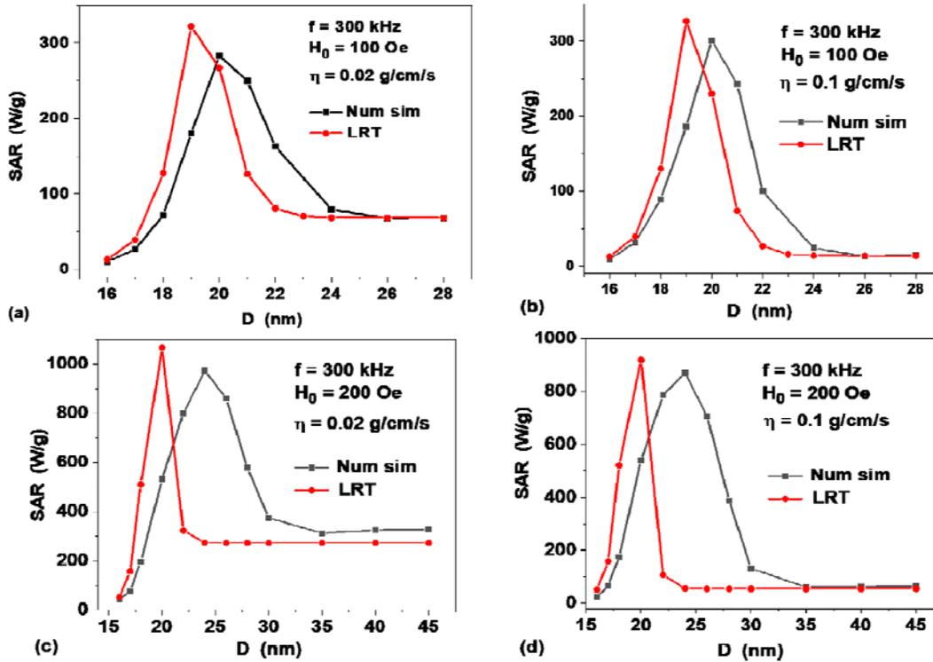
Fig. 5. Comparison of the numerical simulation data and the LRT approximation for different values of the liquid viscosity and the moderate values of ac magnetic field amplitude: a)-b)  $H_0 = 100$  Oe, c)-d)  $H_0 = 200$  Oe.
