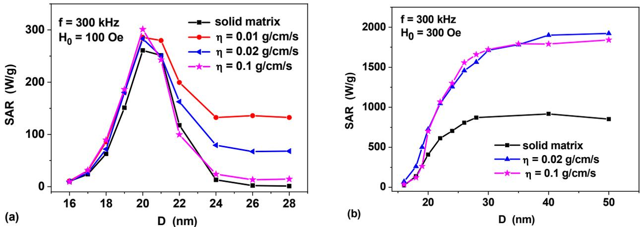
Fig. 6. Comparison of SAR of dilute assemblies of nanoparticles distributed in a solid matrix and in liquids with various viscosity,  $\eta = 0.01 - 0.1$  g/(cm·s) for different amplitudes of ac magnetic field: a)  $H_0 = 100$  Oe, b)  $H_0 = 300$  Oe.
