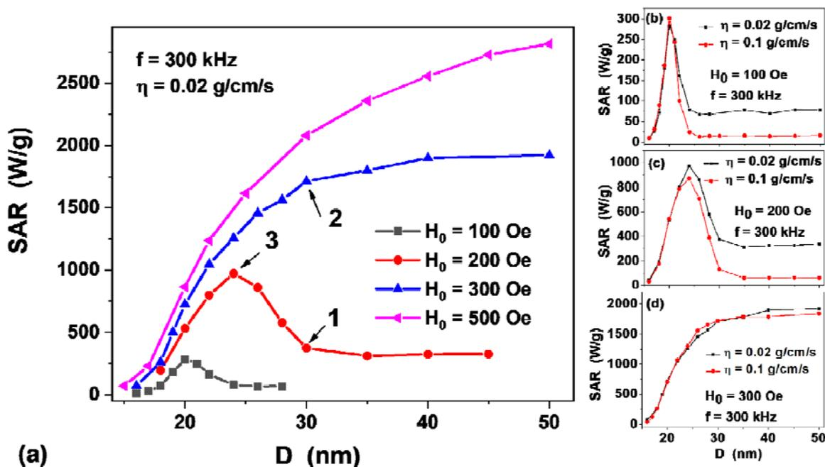
Fig. 1. a) SAR of a dilute assembly of magnetic nanoparticles depending on the particle diameter for different ac magnetic field amplitudes  $H_0$  at the liquid viscosity  $\eta = 0.02 \text{ g}/(\text{cm}\cdot\text{s})$ . b-d) dependence of SAR on the liquid viscosity for various ac magnetic field amplitudes.
