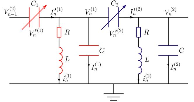
FIG. 12. The unit cell of nonlinear topoelectrical circuit. It is composed of two pairs of  $LC$  resonators of natural frequency  $\omega_0$ , which are connected by nonlinear capacitors  $C_j = C_j(V)$  for  $j = 1, 2$ .
