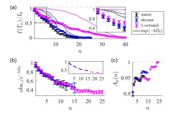
FIG. 4. SG-TIETA  $A_p(n)$  calibration using pure liquids. (a) Observed SG-TIETA decays compared to  $\exp{(-bD_0)}$ .  $D_0$  was measured (see SM Section IV) in legend order as  $2.22\pm0.01, 1.27\pm0.01, 0.121\pm0.002~\mu\text{m}^2/\text{ms}$ . Err. bars =  $\pm1$  SD for 25, 38, 70 repetitions, respectively. (b) Decay vs.  $\exp{(-bD_0)}$  ratio truncated at n=12, 15, 25. Inset shows cubic spline fits. (c)  $A_p(n)$  approximated using adjacent fitted ratios.
