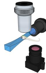
Figure 2: SPIM setup corresponds to the top camera and the lightsheet device, behavior is recorded thanks to the camera represented below the tail.
