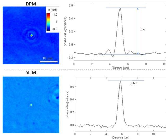
Fig. 2. Oil-immersed, 1  $\mu\text{m}$  diameter polystyrene beads imaged by DPM and SLIM, as indicated. The measured phase values are comparable to the expected number, as detailed in text.
