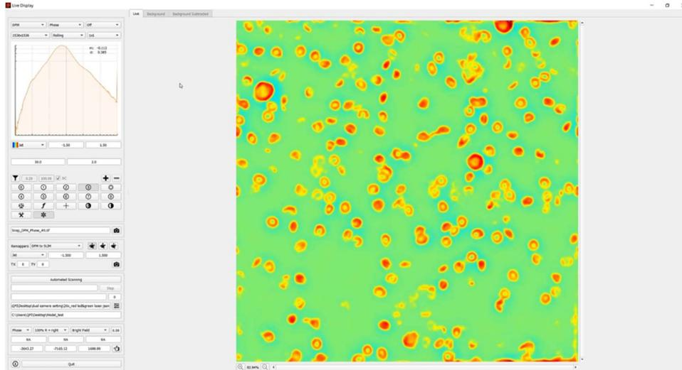
Fig. 6. Live imaging interface. We demonstrate our live imaging system through the three channels: DPM, SLIM, and CIM channel (see Visualization 1). The image shows the graphic user interface and a snapshot of CIM operation in real-time.
