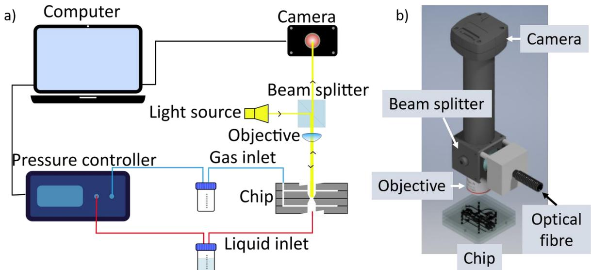
**Figure 2:** a) General setup of the microfluidic thin film pressure balance: a multi-channel pressure controller applies a well-defined capillary pressure to a free-standing film maintained by a bike-wheel type cone in the centre of the microfluidic chip. The film is visualised (and its thickness analysed) using interference of white light reflected from the film and detected by a CCD camera. b) Three-dimensional view of the chip and the optical system.
