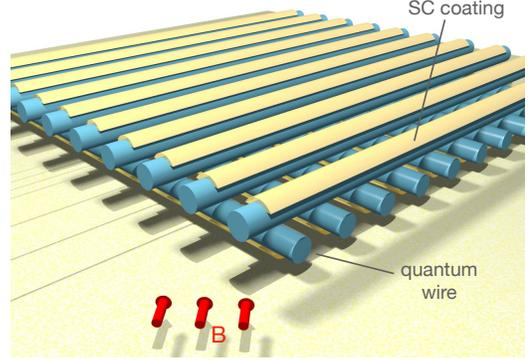
FIG. 1. Geometry of the proposed device. Semiconductor quantum wires coated on one side with a thin layer of conventional superconductor, such as Al, are assembled into two arrays and stacked with twist angle close to  $90^\circ$  as shown.
