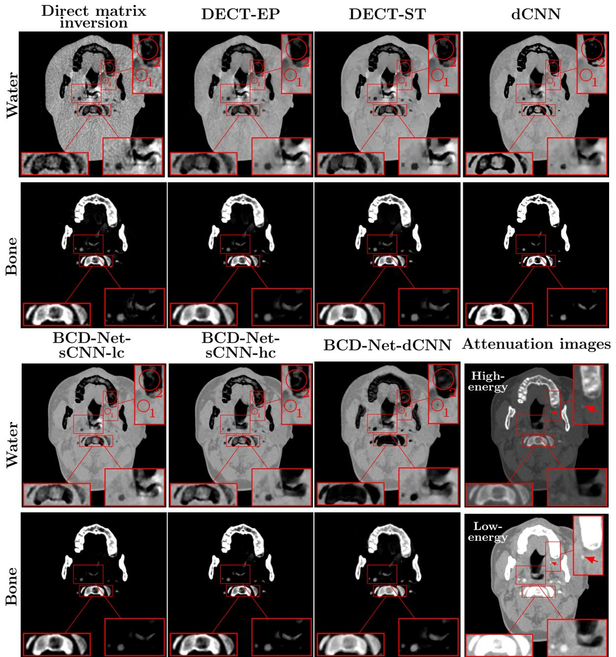
Figure 8: Comparison of decomposed images from different methods (clinical head data). Water and bone images are displayed with windows  $[0.5 \ 1.3] \text{ g/cm}^3$  and  $[0.05 \ 0.905] \text{ g/cm}^3$ , respectively. High- and low-energy attenuation images are displayed with window  $[0.1 \ 0.35] \text{ cm}^{-1}$ .
