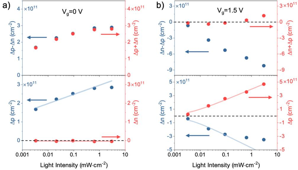
Fig.5 a) Excess electrons and holes found from photo Hall effects and four-probe photoconductance measurements at the gate voltage  $V_g = 0V$ . b) Excess electrons and holes found from photo Hall effects and four-probe photoconductance measurements at the gate voltage  $V_g = 1.5V$ .
