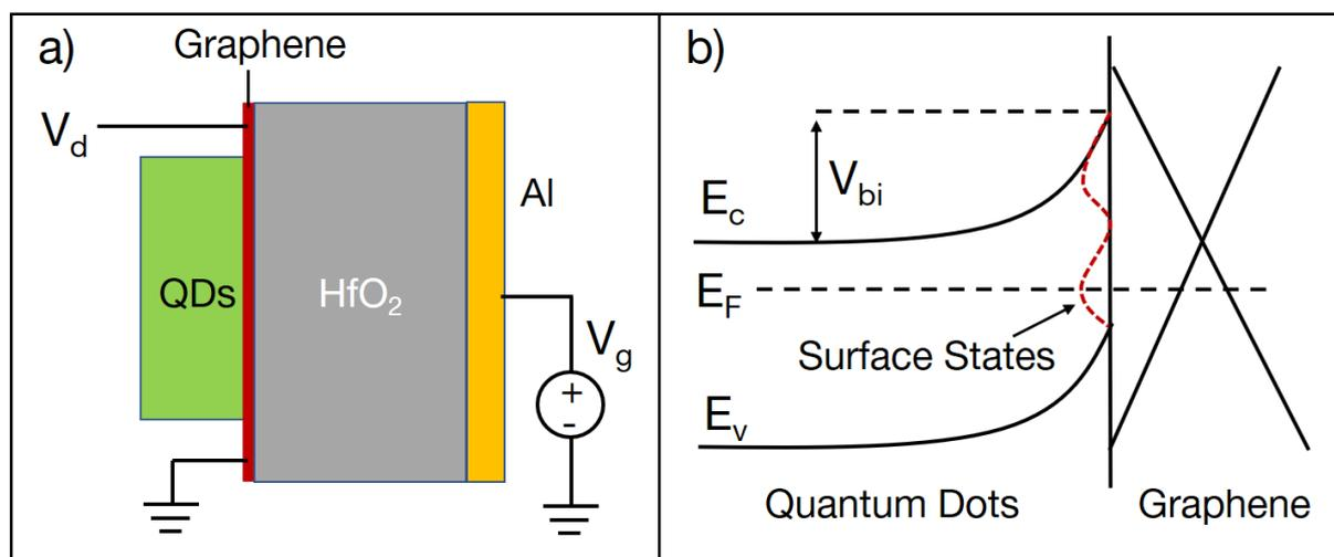
Figure 3 a) Device schematic with quantum dots forming a solid thin film on graphene. b) Energy band diagram of a graphene/QDs device. The energy band in the QDs film bends up towards surface because the work function of the QDs film is smaller than graphene. Electrons will transfer from QDs to graphene after QDs are coated on graphene, which left-shifts the appeared gate transfer characteristics as shown in Fig.1c.
