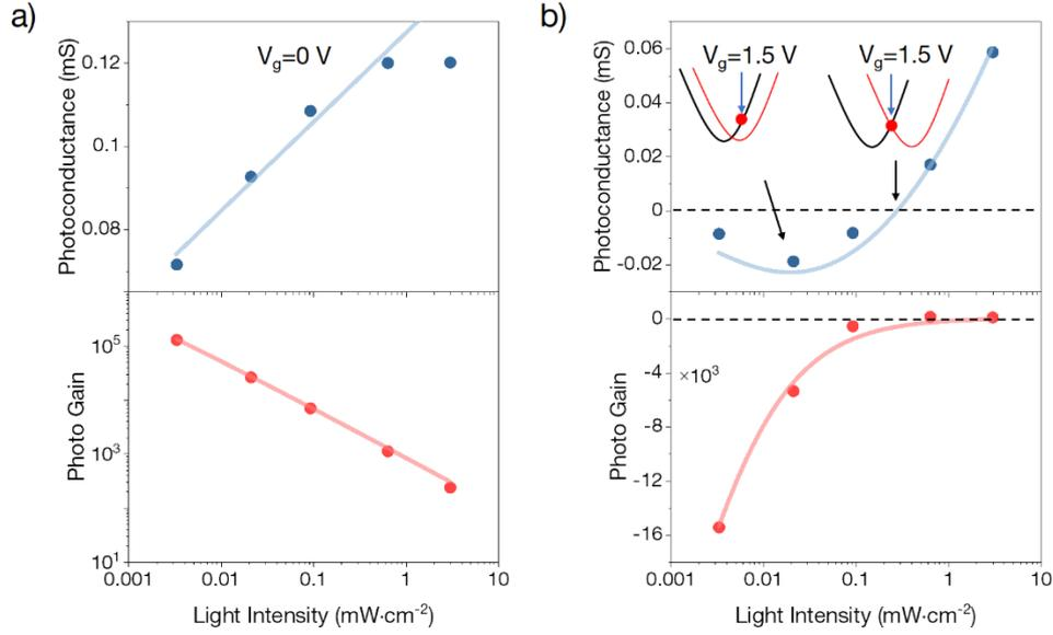
Fig.6 a) Photoconductivity and photo gain at  $V_g = 0\text{V}$ . Dots are experimental data and solid lines in top and bottom panel are fitting lines of theoretical equations eq.(12) and (13), respectively. b) Photoconductivity and photo gain at  $V_g = 1.5\text{V}$ . Dots are experimental data and solid lines in top and bottom panel are fitting lines of theoretical equations eq.(S6) and eq.(S7) in SI Section 3, respectively.
