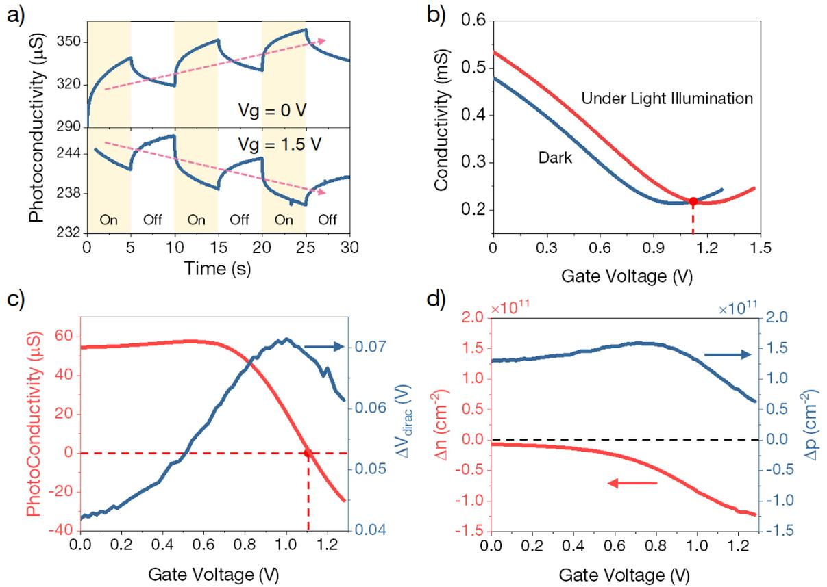
Fig.4 a) Transient photoresponses of graphene/QDs devices upon light illumination that is chopped On/Off. b) Gate transfer characteristics of graphene/QDs device in darkness and under light illumination at the wavelength  $\lambda = 532$  nm and the intensity of  $0.003$  mW/cm<sup>2</sup>. c) Photoconductivity and intrinsic Dirac point shift at different gate voltage. d) Excess holes  $\Delta p$  and electrons  $\Delta n$  as a function of gate voltage.
