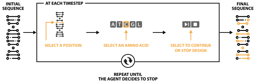
Figure 1: Protein design expressed as a Markovian Decision Process. Figure shows the iterative problem formulation, where the first state is initialized with a sequence to be mutated by the RL agent. Here we depict the sequential action space used by SPPO, where the policy is factorized over the decisions of which position to select, what to change it to, and when to stop mutating.
