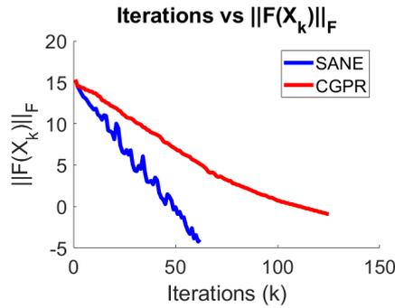
(b) Iterations vs  $\|F(X_k)\|_F$ **Fig. 2** Averaged convergence history of RSANE and CGPR, from the same initial point, for the joint diagonalization Riemannian gradient vector field. On the left,  $(n, p, N) = (500, 100, 5)$ , and on the right  $(n, p, N) = (1000, 100, 5)$ . The y-axis is in logarithmic scale.
