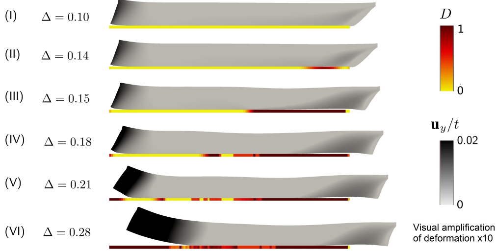
Figure 6: Peeling sequence for layer with l/t = 12 and parameter values in (15). The imposed displacement is increased from (I) to (VI). At every stage, the (magnified) deformation of the layer is shown. Grey shading represents vertical displacements. The shaded line at the bottom of the layer represents the level of damage of the cohesive elements in their undeformed location. Formation of an interfacial cavity (II), and subsequent shedding of a smaller cavity (IV) are shown as reattachment occurs. Finally, curling becomes noticeable and ultimately leads to complete failure (VI).
