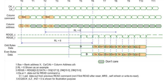
Fig. 4: Read access timing from JESD235C. The access starts with the first read request to column address Ca. After R T-cycles (T0 to T6 for R=6 example) a burst of 4 128-bit words, Da to Da+3, is available on DQ[127:0]. Similarly, the second read request to column address Cb generates a burst of 4 128-bit words, Db to Db+3. The DPR-BUF combines the 8 128-bit words and writes them into 8 corresponding FIFOs. The 8 FIFOs are then read into the 1024 bit on-chip buffer.
