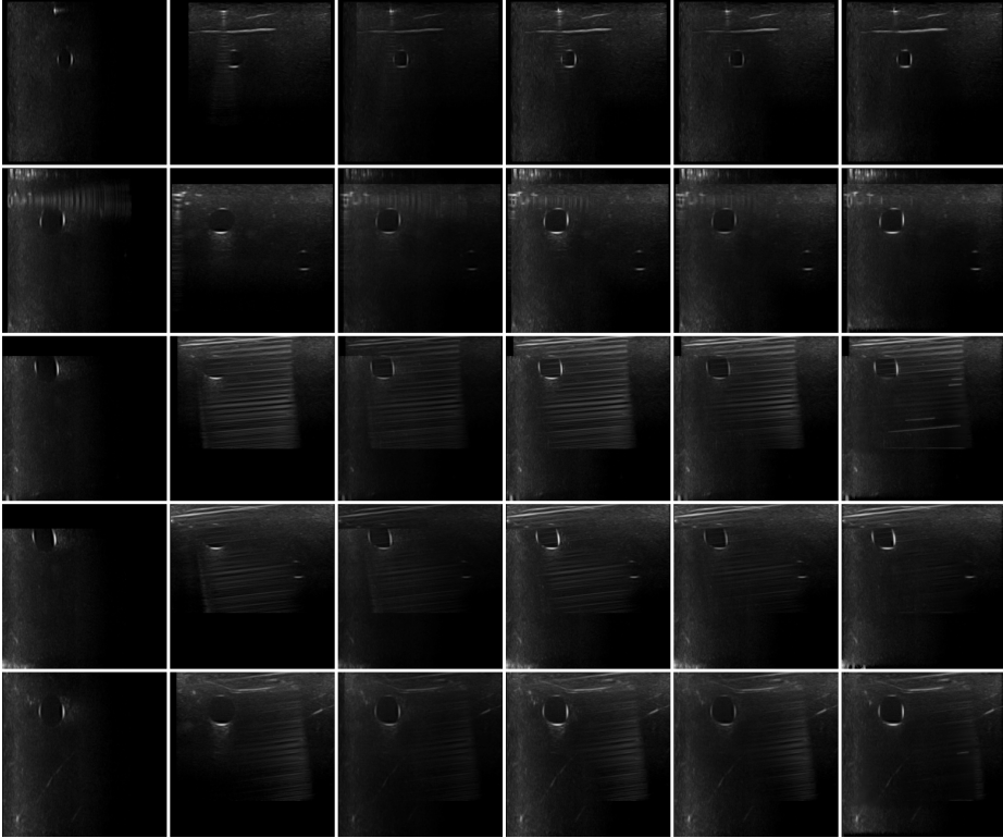
Fig. 5: Results on the phantom with a needle inserted in it. The left two columns are the two input images (phantom images were acquired orthogonally within plane, where the imaging direction of the first and second column are from left to right and from top to bottom respectively). The right four columns from left to right are results from average [33], maximum [18], uncertainty-based fusion [4], and our algorithm. On the phantom examples it is clear that our method best preserves bright and dark anatomy while suppressing artifacts.
