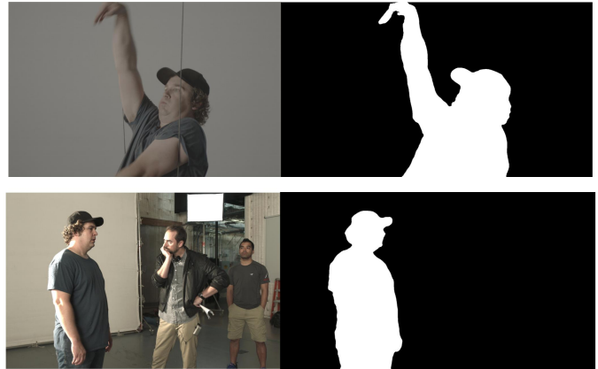
Figure 8: Example HyperSeg segmentation outputs from test data taken from the VFX Segmentation dataset (10 total clicks).
