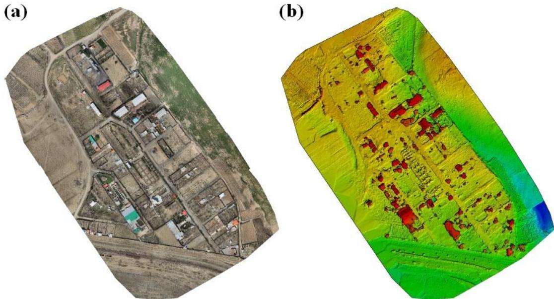
Figure 6. Products generated from Pix4Dmapper, (a) orthomosaic, and (b) digital surface model (DSM) with average ground sampling distance (GSD) equal to 1.91 cm.
