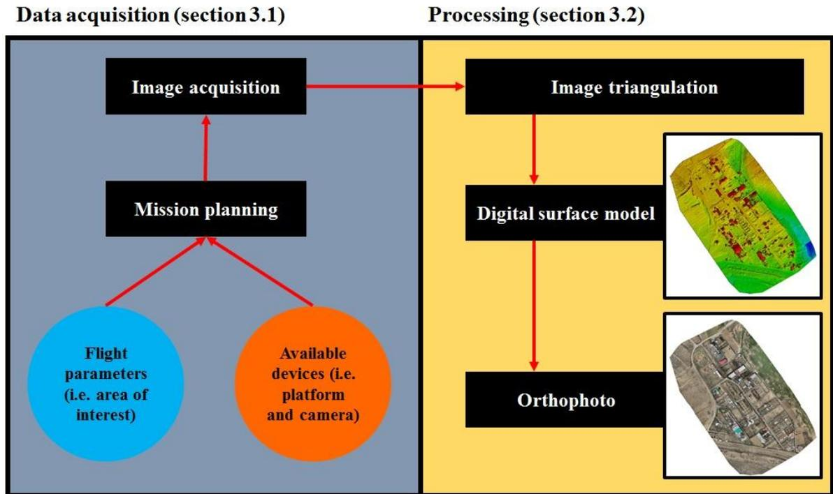
Figure 3. Workflow schematic as for evaluating the SAMA-VTOL.
