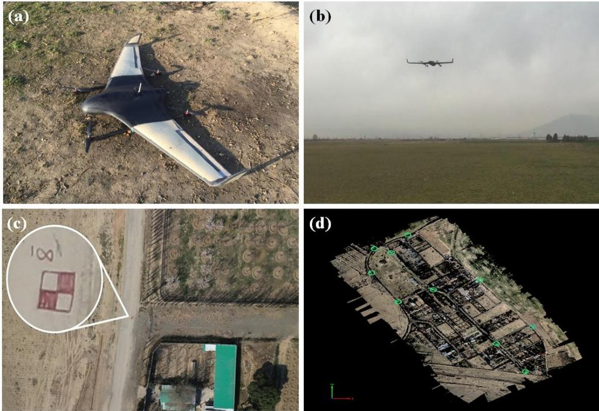
Figure 5. Overview of the research equipment, (a) SAMA-VTOL equipped with CANON EOS M digital camera, (b) SAMA-VTOL taking off, (c) checkpoint template, and (d) distribution of checkpoints.
