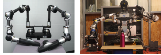
Fig. 1: Robot Hardware used in the study. The Imitation Controller (left) is a scaled kinematic replica of the robot (right).
