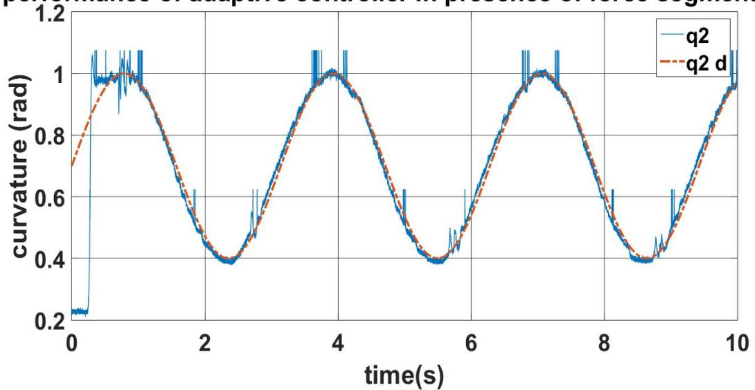
Figure 5.7: Adaptive controller tracking for lower actuator in interaction with the environment
