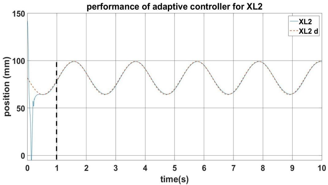
Figure 7.5: Performance of locked control system in vertical direction
