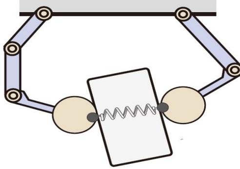
Figure 7.3: Assuming an imaginary spring for generating gripping force [7]
