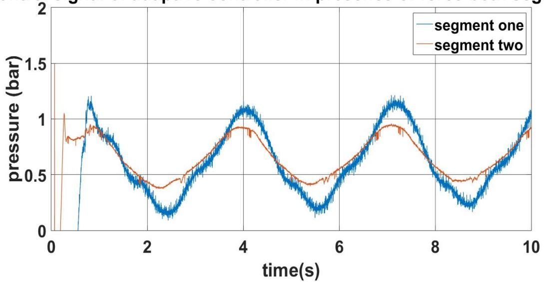
Figure 5.8: Control effort for both actuators in tracking the desired trajectory by adaptive controller in interaction with the environment
