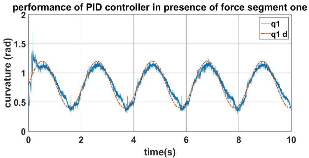
Figure 5.14: PID controller tracking for upper actuator in interaction with the environment
