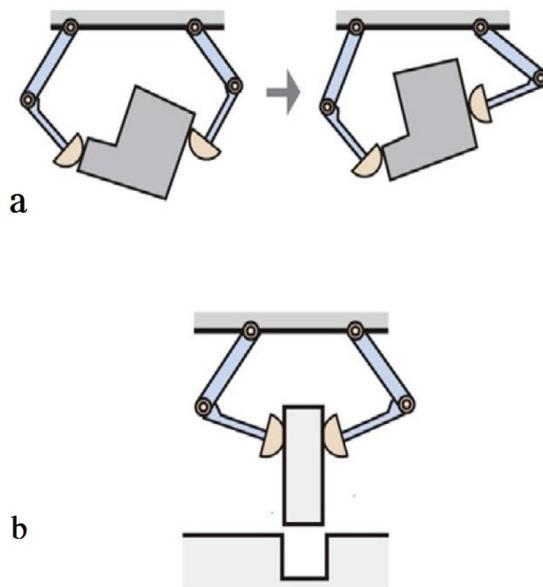
Figure 1.2: Performing in-hand object manipulation [2]. Changing the a) orientation b) position of the object
