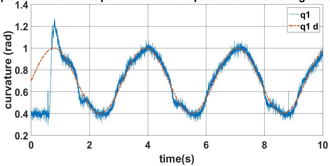
Figure 5.6: Adaptive controller tracking for upper actuator in interaction with the environment
