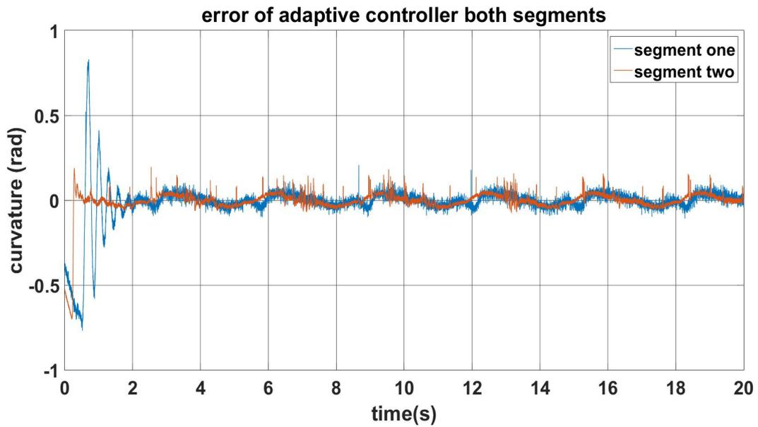
Figure 5.3: Error of tracking the reference trajectory through adaptive controller for both actuators
