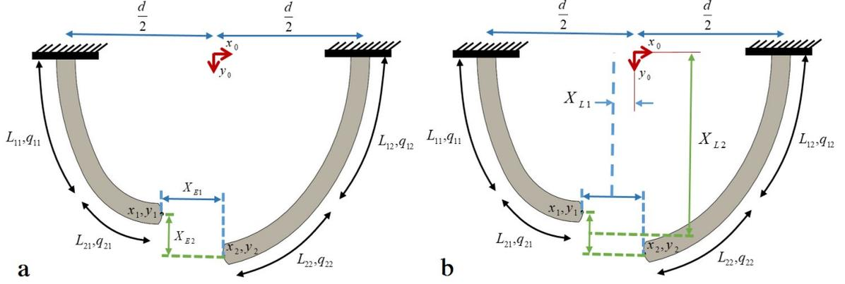
Figure 7.2: Defining shaped and locked variables for two-fingered soft gripper
