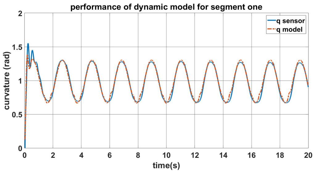
Figure 4.4: Accuracy of dynamic model for upper bending actuator as a response to pressure  $0.8 + 0.4\sin(3t)$
