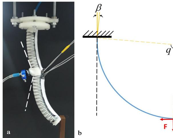
Figure 6.3: Effect of external force a) on two-segmented soft finger. b) on a single bending actuator [5]
