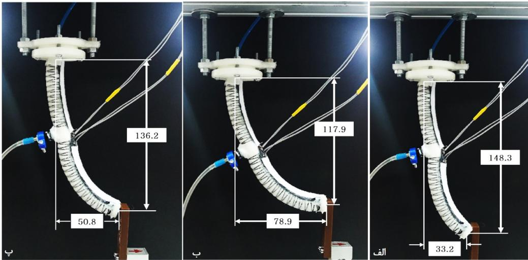
Figure 6.1: Obtaining the tip position of soft finger while measuring the force by load cell
