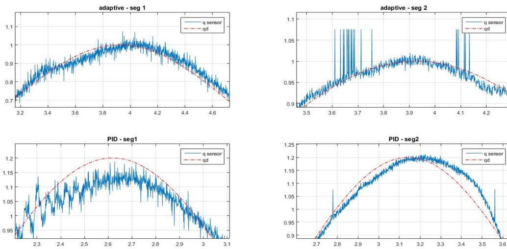
Figure 5.19: Comparing the performance of PID and Adaptive controllers in interaction with the environment for both actuators
