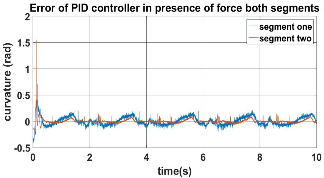
Figure 5.16: Error of tracking the reference trajectory through PID controller for both actuators in interaction with the environment
