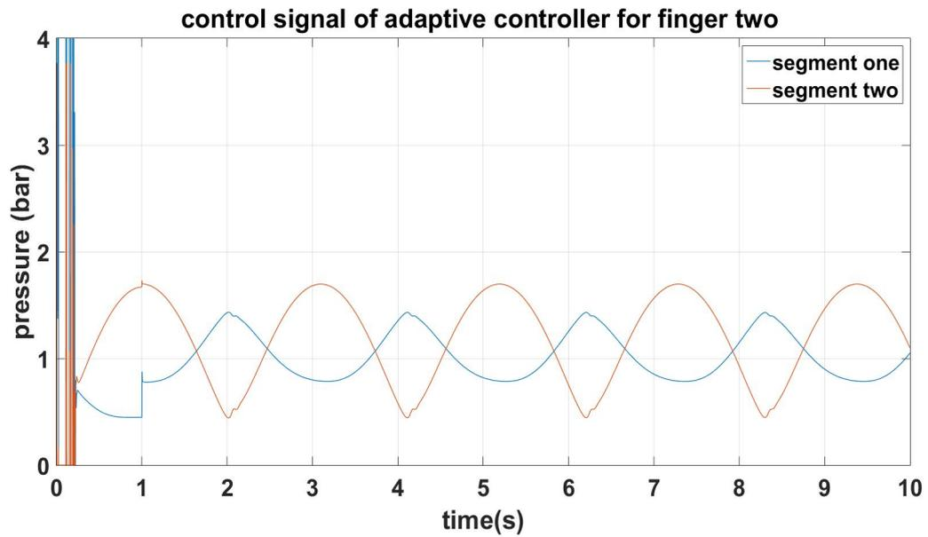
Figure 7.9: Control pressure for soft finger two in shaped and locked system
