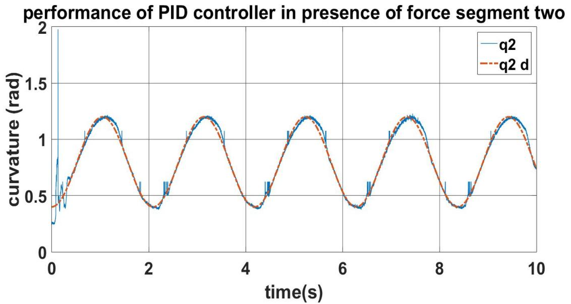
Figure 5.15: PID controller tracking for lower actuator in interaction with the environment
