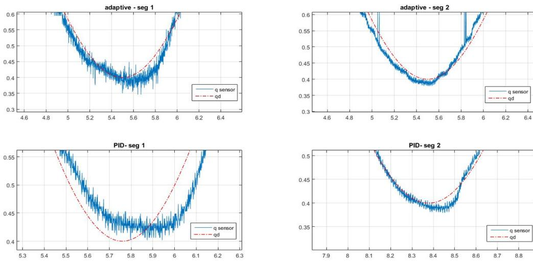
Figure 5.18: Comparing the performance of PID and Adaptive controllers in free motion for both actuators
