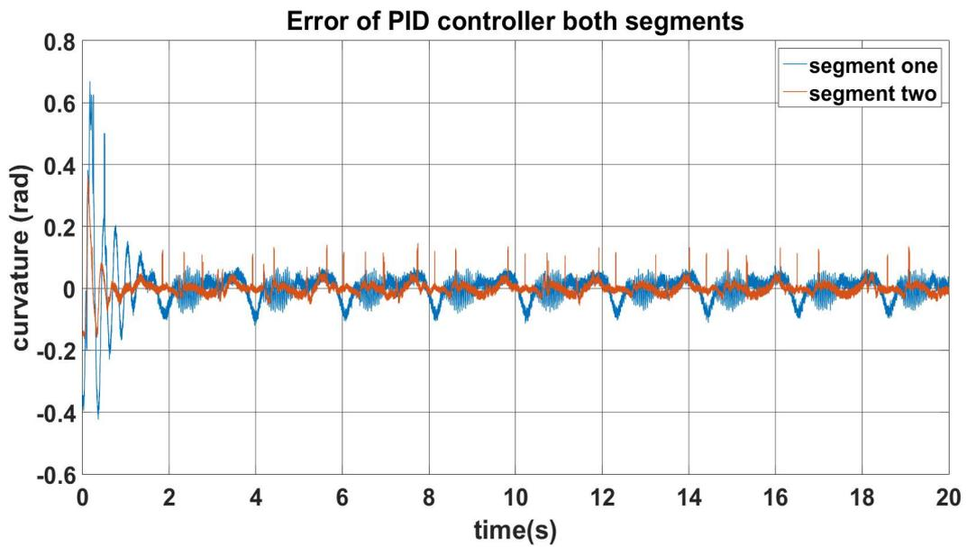
Figure 5.12: Error of tracking the reference trajectory through PID controller for both actuators
