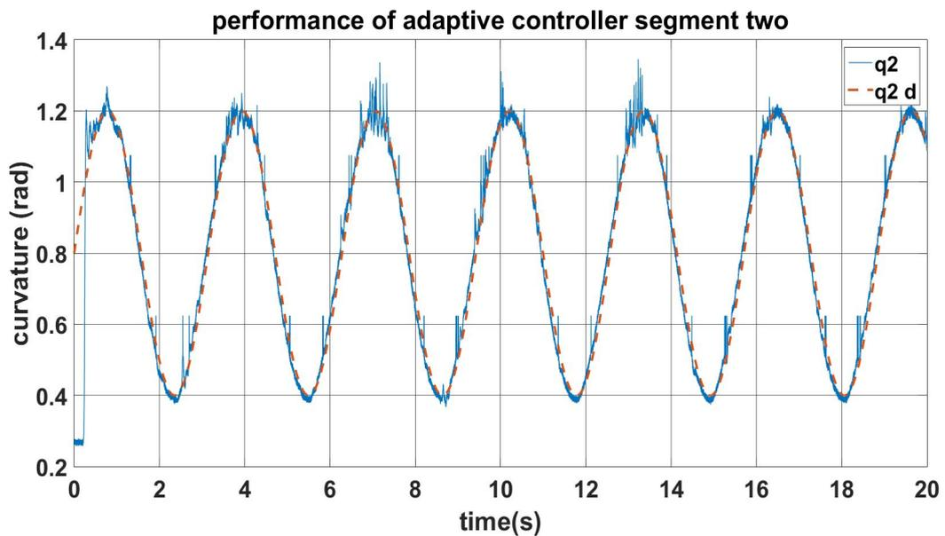
Figure 5.2: Tracking the reference trajectory by lower bending actuator through adaptive controller
