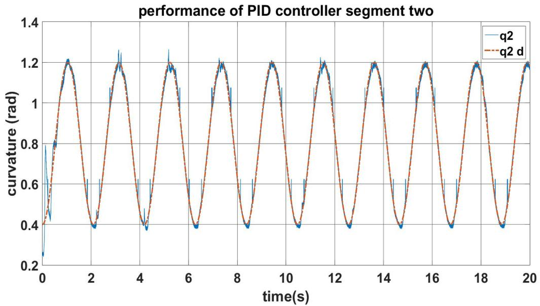
Figure 5.11: Tracking the reference trajectory of lower bending actuator by PID controller
