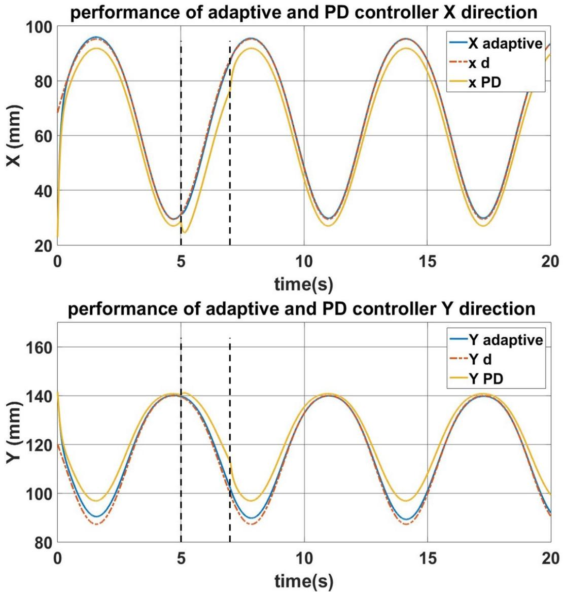
Figure 6.5: Performance of adaptive controller in response to kinematic and dynamic uncertainties in comparison to performance of feed back linearization controller
