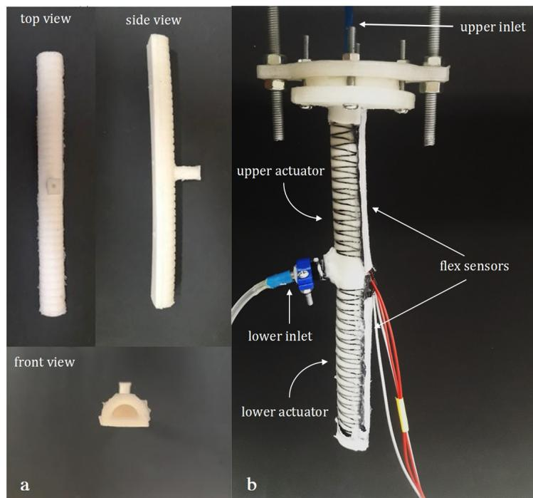
Figure 3.2: Fabricated soft finger. a) Three main views of molded rubber body. b) Different parts of the soft finger
