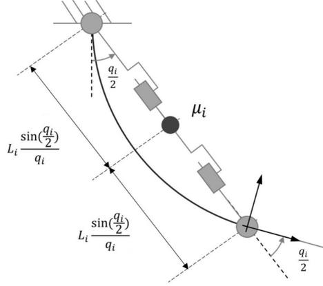
Figure 4.2: Single bending actuator and proposed equivalent rigid manipulator [4]
