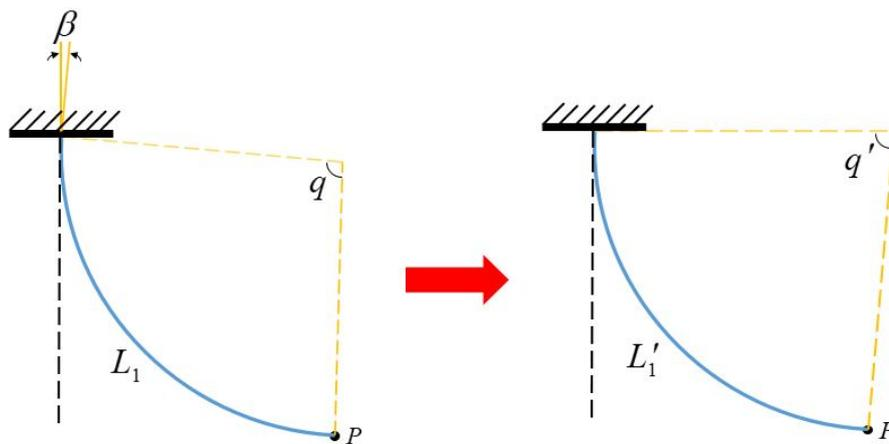
Figure 6.4: Reaching to the same position without deflection by appropriate estimation of length and curvature
