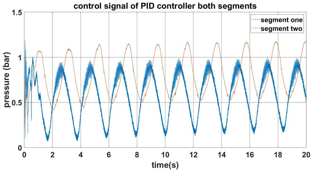
Figure 5.13: Control effort for both actuators in tracking the desired trajectory by PID controller
