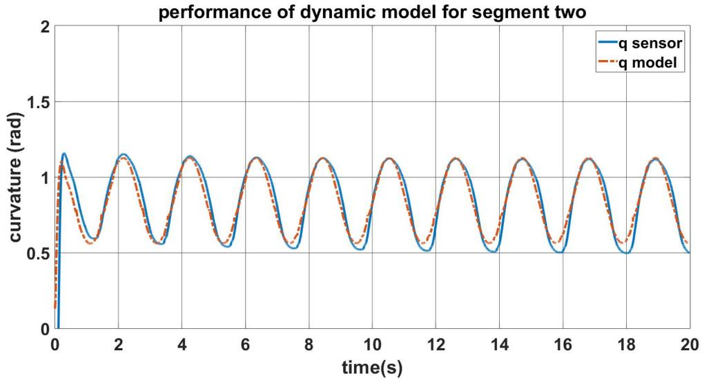
Figure 4.5: Accuracy of dynamic model for lower bending actuator as a response to pressure  $0.8 + 0.4\sin(3t + 1.57)$
