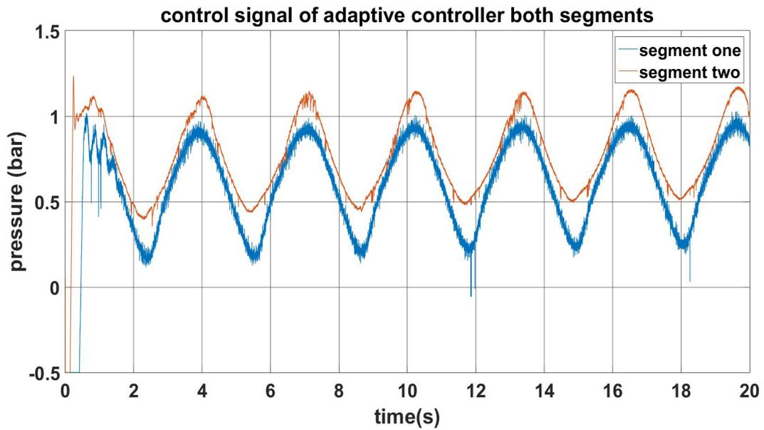
Figure 5.4: Control effort for both actuators in tracking the desired trajectory by adaptive controller
