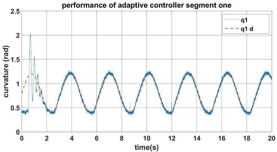
Figure 5.1: Tracking the reference trajectory of upper bending actuator by adaptive controller
