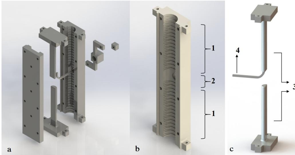
Figure 3.1: Proposed mold for fabrication of soft fingers. a) its components and how they are assembled. b) Staple component of the mold. c) half-round rods to define interior hallow portions of the actuators.
