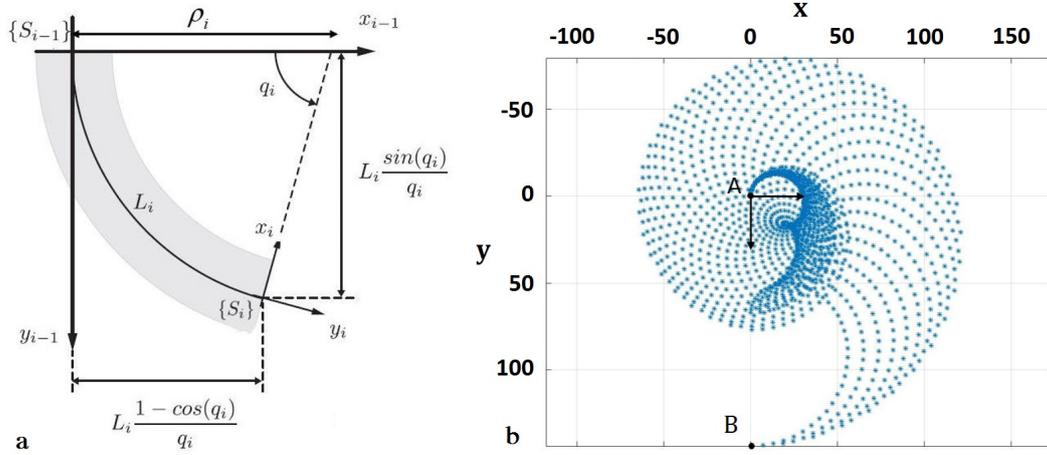
Figure 4.1: a) Single bending actuator planar bending [3]. b) Work space of the two-segmented soft finger for 360 degree bending of each actuator.
