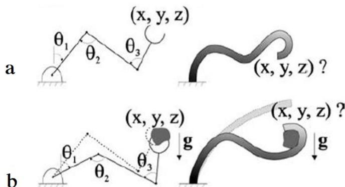
Figure 1.1: Soft robotics' challenges in comparison to conventional robotics [1] a) infinite degree of freedom b) greater impacts of external forces
