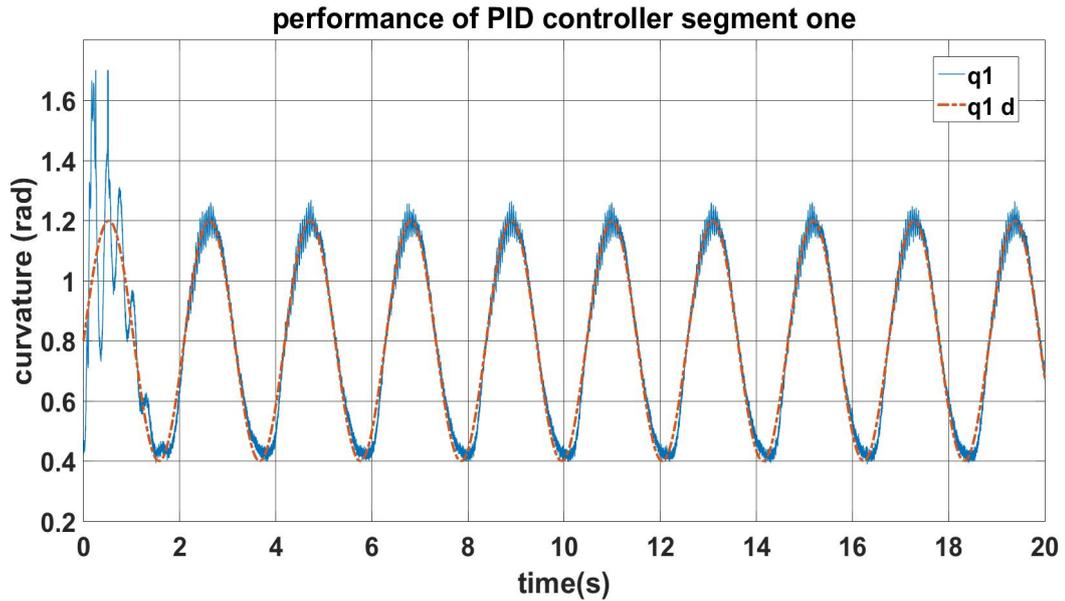
Figure 5.10: Tracking the reference trajectory of upper bending actuator by PID controller
