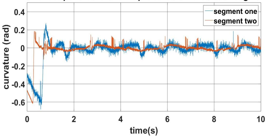
Figure 5.9: Error of tracking the reference trajectory through adaptive controller for both actuators in interaction with the environment
