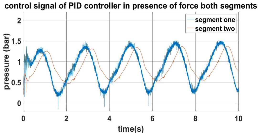
Figure 5.17: Control effort for both actuators in tracking the desired trajectory by PID controller in interaction with the environment
