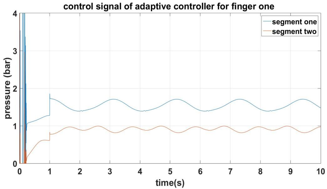
Figure 7.8: Control pressure for soft finger one in shaped and locked system
