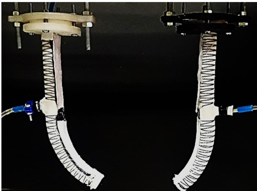
Figure 1.3: Proposed two-fingered gripper
