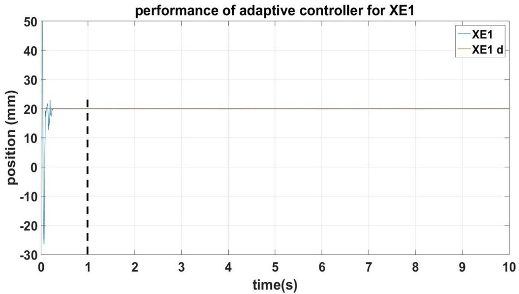
Figure 7.6: Performance of shaped control system in horizontal direction
