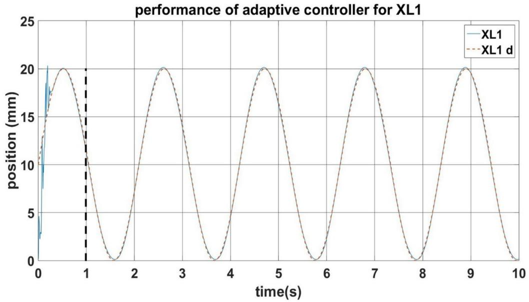
Figure 7.4: Performance of locked control system in horizontal direction
