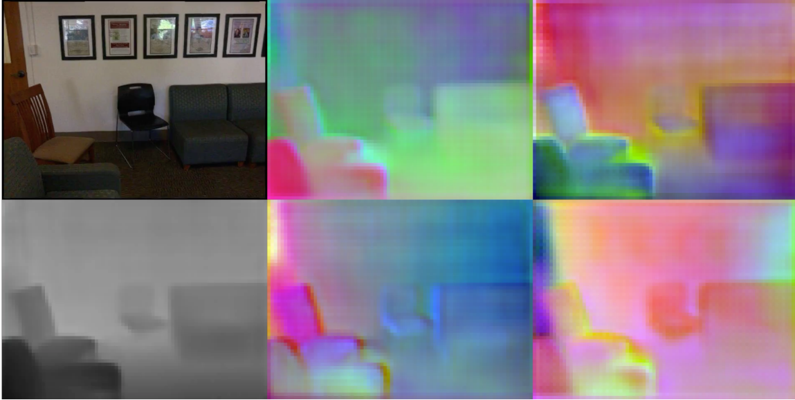
Figure 5: The depth prediction network Top left: an input image. Bottom left: the predicted depth. Middle and right: We use SVD to reduce the 32 factors-of-variation planes down to 12 planes, and display them as 4 RGB images; each of the 4 \times 3 color planes represents one factor of variation.
