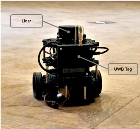
Fig. 3: The robotic platform used for the experimentation: a Robotis TurtleBot3 Burger with a Decawave EVB1000 Ultra-wideband tag.
