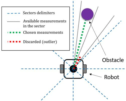
Fig. 2: Scheme of used lidar measurements. Lower values of distance are considered more significant for obstacle detection.
