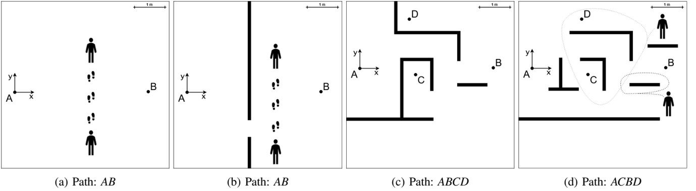
Fig. 6: Scenarios used in the second set of tests for the comparison with human control. Points positions:  $A(0,0)$  m,  $B(4.45,0.02)$  m,  $C(1.86,-0.21)$  m,  $D(1.65,1.65)$  m.
