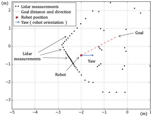
Fig. 7: Human interface during the second tests set. Testers are allowed to see lidar measurements, robot pose and goal distance and direction.
