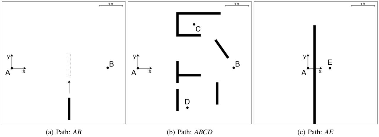
Fig. 4: Scenarios used in the first set of tests for the local planner evaluation. Points positions:  $A(0,0)$  m,  $B(4.35,0.02)$  m,  $C(2.55,2)$  m,  $D(2.25,-1.8)$  m,  $E(1,0)$  m.
