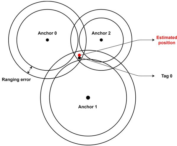
Fig. 5: Estimation of the position in the x-y plan using error affected ranging measurements.
