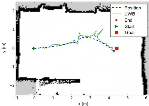
Fig. 8: Trajectory followed in a test in the first scenario (path  $AB$ , interrupted by a sudden moving person). The UWB added noise is clearly visible and shows how the proposed local planner is highly robust against positioning errors.
