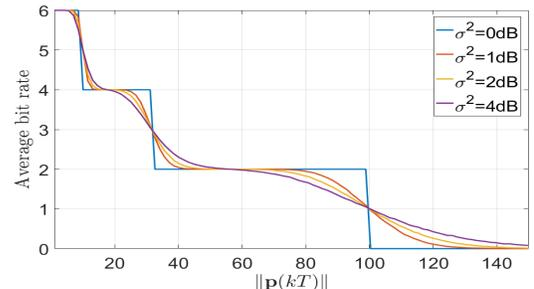
Figure 1. Average bit rate  $\mathbb{E}[R(\Gamma(\mathbf{p}(kT)))]$  for  $R_0 = 0$ ,  $R_1 = 2$ ,  $R_2 = 4$ ,  $R_3 = 6$ ,  $\eta_1 = 0.001$ ,  $\eta_2 = 0.01$ ,  $\eta_3 = 0.1$ ,  $\alpha = 2$  and different shadowing variances.
