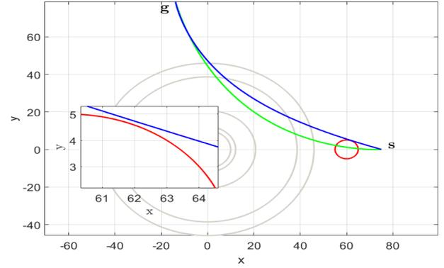
Figure 5. Paths corresponding to the optimum trajectories ( $\lambda = 0.6$ ) considering the obstacle (blue) and without considering the obstacle (green). The magnified image shows the vicinity of the obstacle.
