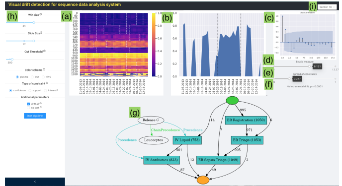
Figure 6: The user interface of the VDD system, running on the Sepsis event log [1]. (a) Drift Map. (b) Drift Chart. (c) Autocorrelation plot. (d) Erratic measure. (e) Spread of constraints view. (f) Incremental drifts test. (g) Extended Directly-Follows Graph. (i) Behavior cluster selection menu.
