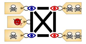
**Figure 11.** Failure Disagreement Learner Graph: Learners are shown as eyes, with darker blue learners on the left, and lighter, outlined red learners on the right. The edge between the blue learners is labeled with one Byzantine failure: they want to agree even if one acceptor is Byzantine. All the other learners may disagree if there is a Byzantine failure. The learners are each labeled with a number of crash failures: they want to terminate even if one or two acceptors crash.
