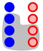
**Figure 7.** Heterogeneous Failures and Acceptors Example: Here, we draw one group of acceptors as solid blue circles, and the other as hollow red circles. A quorum is shown as a shaded region.
