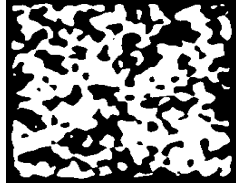
Fig. 6: Example of the high-contrast coefficients for the variable-coefficient Poisson's equation in the unit square with a 2D grid 256 \times 256 .
