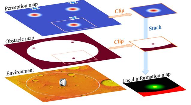
Fig. 3. An example for an information map that is stacked by a perception map and a obstacle map. The state representation is a local information map centered on each drone with size  $2R_s \times 2R_s$ .
