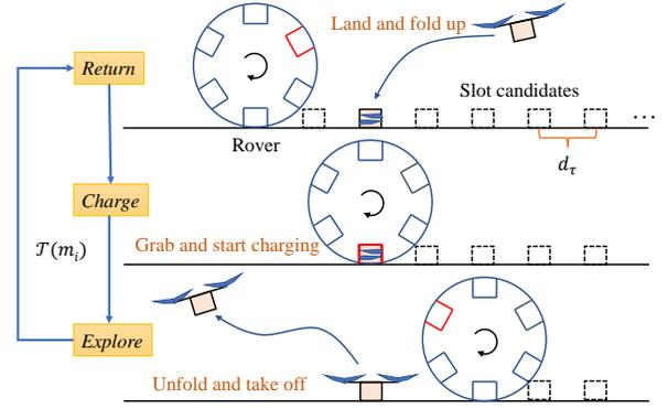
Fig. 4. Illustration of the charging process and switching between different operating modes.
