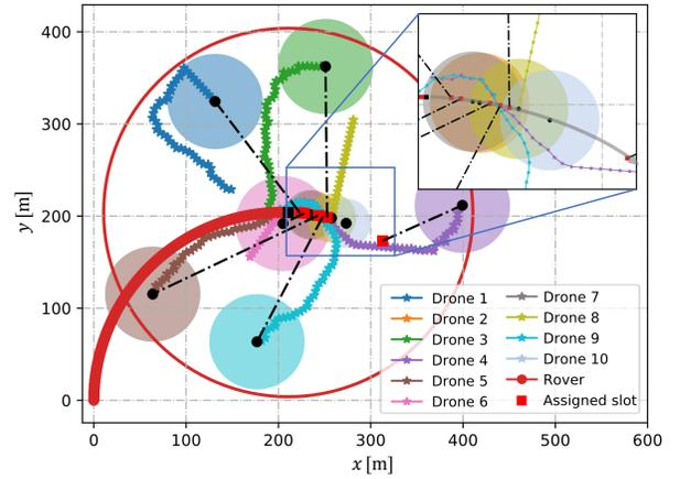
Fig. 6. A snapshot of drone trajectories at  $t = 650$  s. The dashed lines are used to connect drones with currently assigned charging slots. We use large circles to represent drones under exploration, and small circles to represent drones parked in the charging slots.
