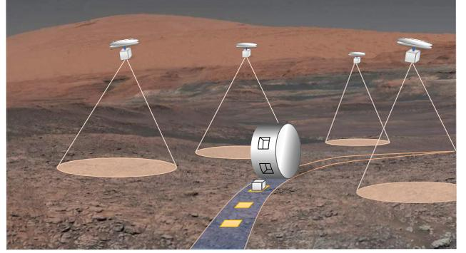
Fig. 1. Conceptual layout of our cooperative Mars exploration system. We evenly arrange several charging slots on the circumference of the rover. Each drone can be recharged by landing on the ground, folding up, and letting the rover roll over it. (The background image was taken by the rover Curiosity.)
