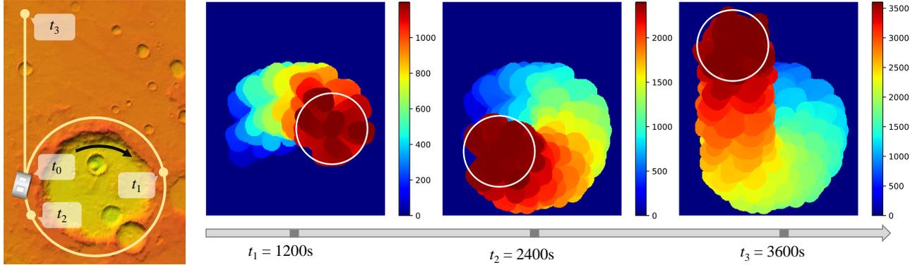
Fig. 5. The designed rover path and snapshots of multi-drone coverage areas ( $n = 10$ ). The mission begins at  $t_0$ , where the drones depart from the rover in turn, and ends at  $t_6 = 3600$  s. The color intensity in each coverage map is positively correlated with time, and we use a white circle to indicate the feasible area for drones.
