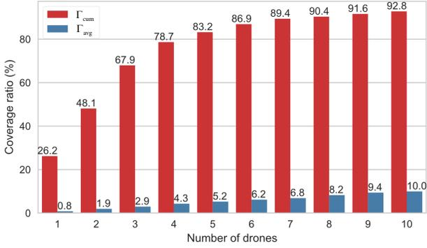
Fig. 7. Comparison of the cumulative coverage ratio  $\Gamma_{cum}$  and the average instantaneous coverage ratio  $\Gamma_{avg}$  under different numbers of drones.
