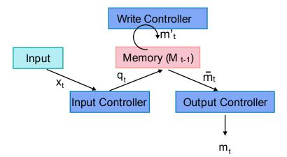
Figure 2: Overview of an external memory which is composed of input, output and write controllers. The input controller determines what facts within the input are used to query the memory. The output controller determines what portion of the memory is passed as the output for that query. Finally the write controller updates the memory state and propagates it to the next time step.
