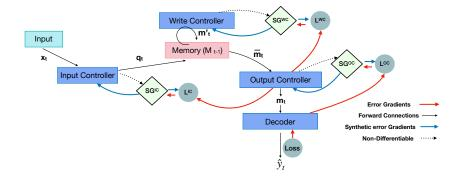
Figure 3: Proposed Framework for Incorporating Synthetic Gradients into the Memory Controllers. The gradient predictor,  $SG^{IC}$ , of the Input Controller, IC, predicts the loss of ICfor its output  $q_t$ . This additional feedback path is utilised by the IC to dynamically adjust its behaviour to different tasks at hand. Similarly, we define gradient predictors,  $SG^{OC}$ , and  $SG^{WC}$ , for output and write controllers respectively.
