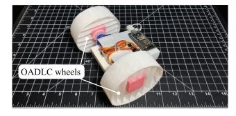
Fig. 7. A foldable car with OADLC wheels, proving the design paradigm can be applied to build circular OADLC mechanisms with in-plane stiffness specification as a design constraint. The width of the square grid is 12.7 mm.
