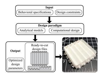
Fig. 1. The flow chart of our computational design and fabrication of OADLC mechanisms. The width of the square grid is 12.7 mm.
