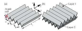
Fig. 2. Corrugated mechanisms with triangular unit cell. (a) A single-layered corrugated sheet with it geometry parameters and coordinate system labeled. (b) A typical OADLC mechanism.
