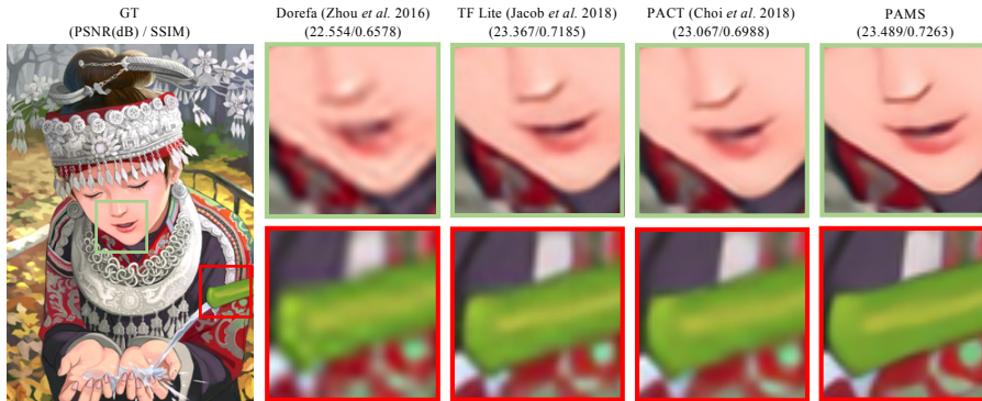
Fig. 4. Qualitative comparison of our method with other quantization methods on a scale factor of \times 4 .
